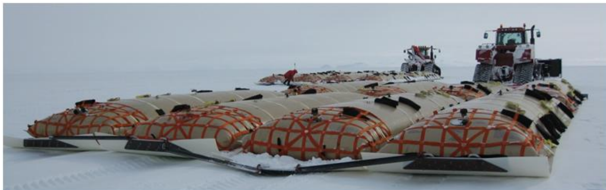
Figure 1. Two SPoT09-10 tractors setup each to haul eight 3000-gal. fuel bladders on four flexible plastic sleds 1030 miles from McMurdo to South Pole.
