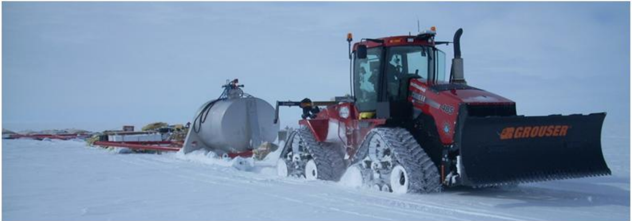
Figure 3. Case Quadtrac towing all GrIT08 heavy sleds: a steel fuel tank, two flexible cargo sleds on a spreader bar and four flexible bladder sleds on a spreader bar. Note high sinkage of the Case rear tracks (~ 12 in.) owing to soft snow and high towing resistance.
