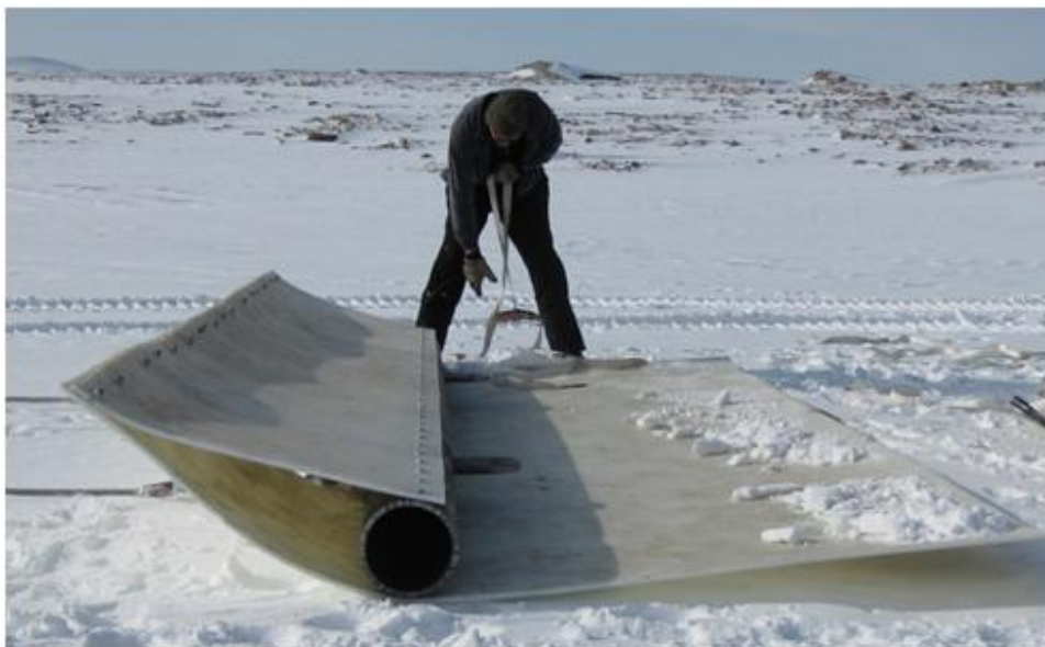
Figure 8. Smaller (16-ft-wide) spreader bar used to shuttle the two bladder sleds through the transition.
