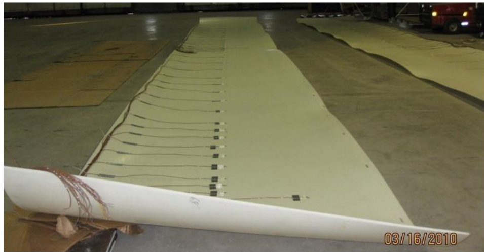
Figure 6. Thermocouples (23 per bladder) installed along the length of each bladder sled. Thermocouple sensing junctions were flush with the bottom surfaces of the sleds. Air temperature, bladder fuel temperatures and solar irradiance were also measured.
