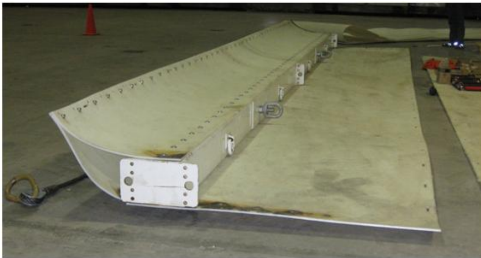
Figure 7. Ski-nose spreader bar for connecting the full sled load (two dual-bladder sleds and Dura-Base cargo sled) to the Case.
