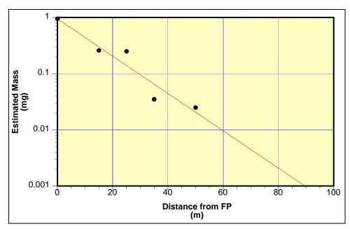
Figure 16. Exponential curve fit for FP residues (●): Case 2.
