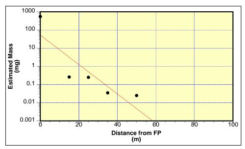
Figure 15. Exponential curve fit for FP residues (●): Case 1.
