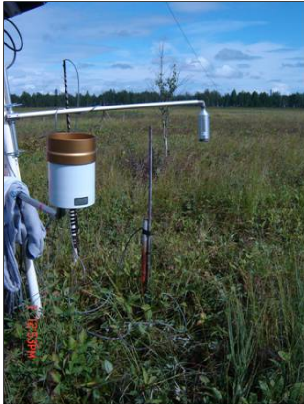
Figure 8. Tipping bucket rain gauge (left) and sonic sounder (right) at Murphy station, August 2007.
