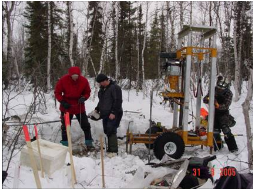
Figure 17. Developing and collecting initial water samples from the Birch Island Well, March 2005.
