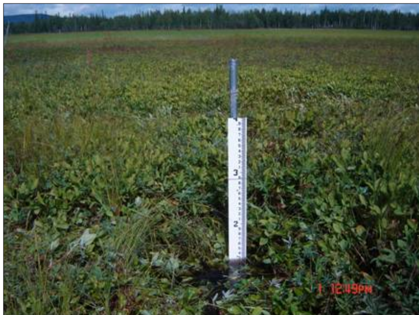
Figure 9. Staff gauge at Murphy station for daily (May–September) water level measurement and posting with a web camera.
