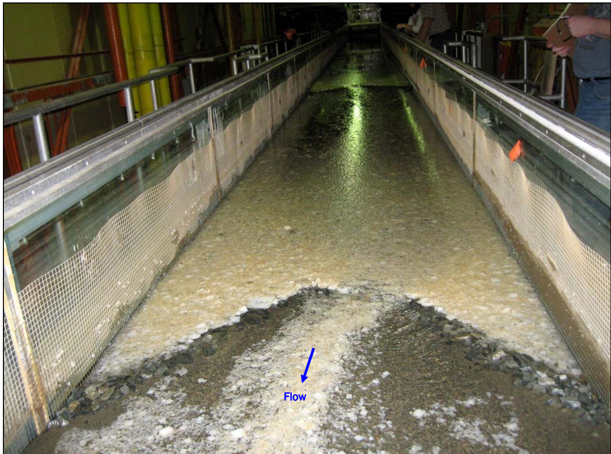
Figure 9. Physical model tests of ice passage over cross vanes in the CRREL flume.
