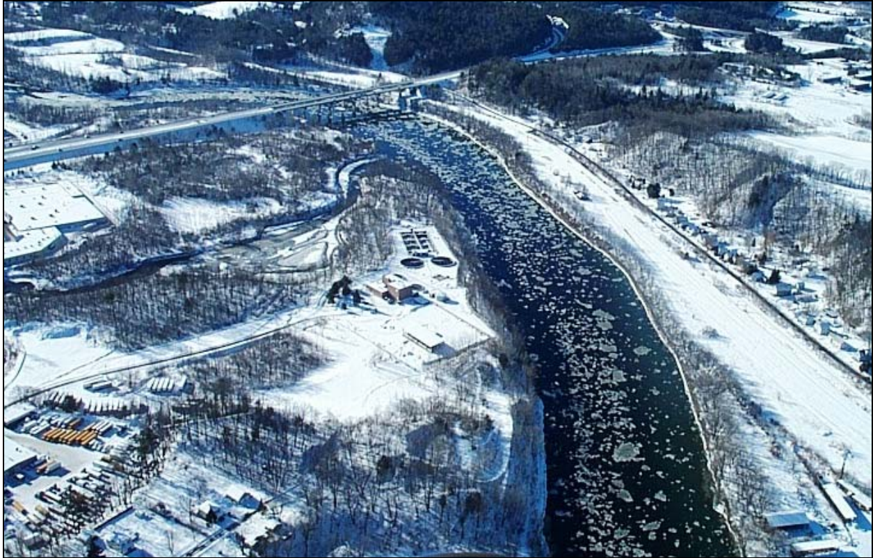
Figure 3. Drifting frazil ice pans on the Kennebec River upstream of Augusta, Maine.
