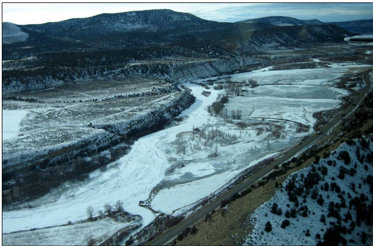
Figure 4. Freezeup ice jam and flooding on the White River downstream of Meeker, Colorado.
