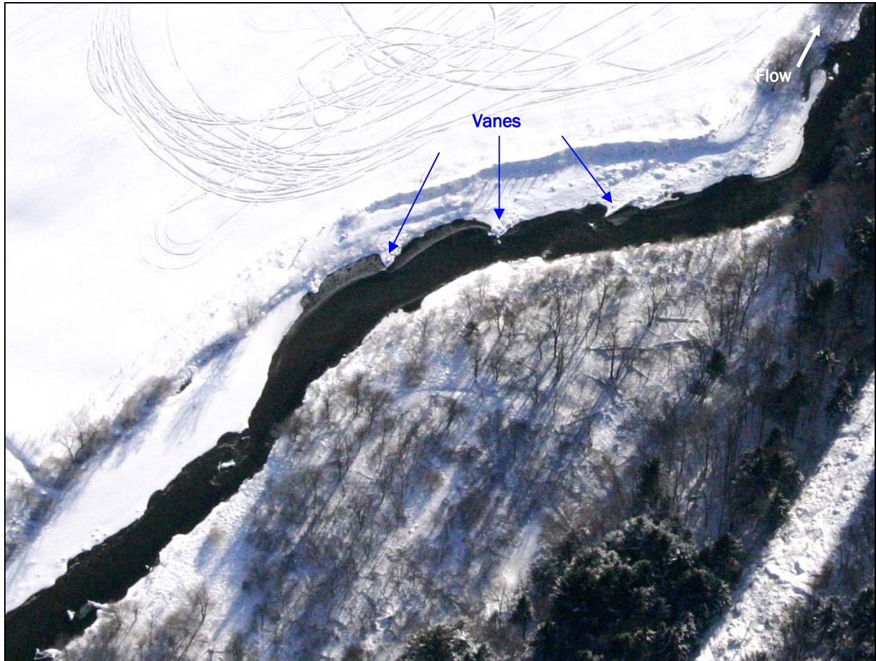
Figure 7. Border ice growth along rock vanes on the White River, Vermont.
