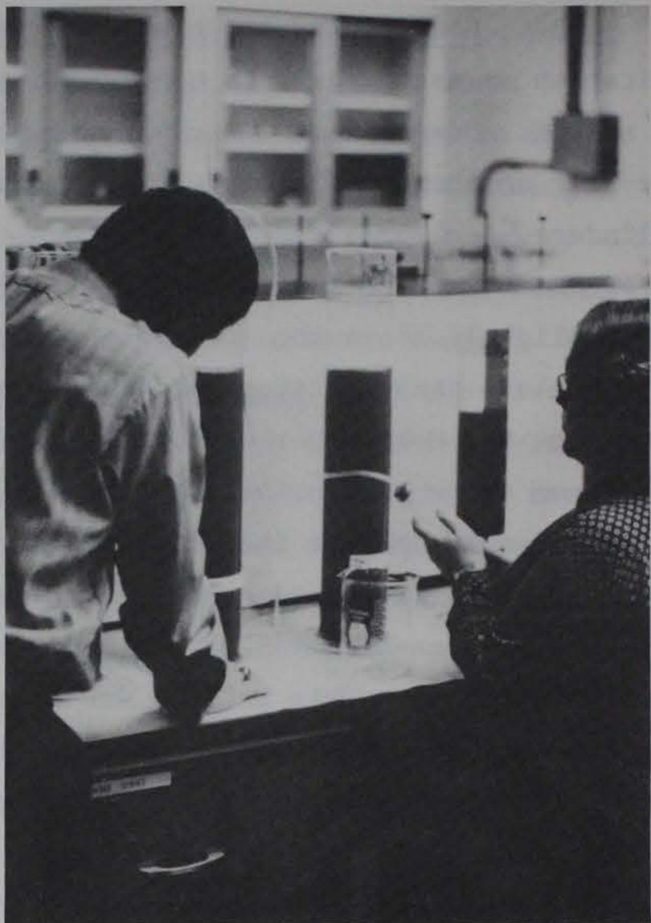
Figure 21. Sample extraction in progress using syringe and tubing
