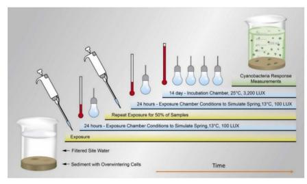
Figure 4. Example of a laboratory method designed to predict algaecide efficacy for overwintering cyanobacteria (reproduced from Calomeni et al., "Efficacy of Algaecides," 2023).
