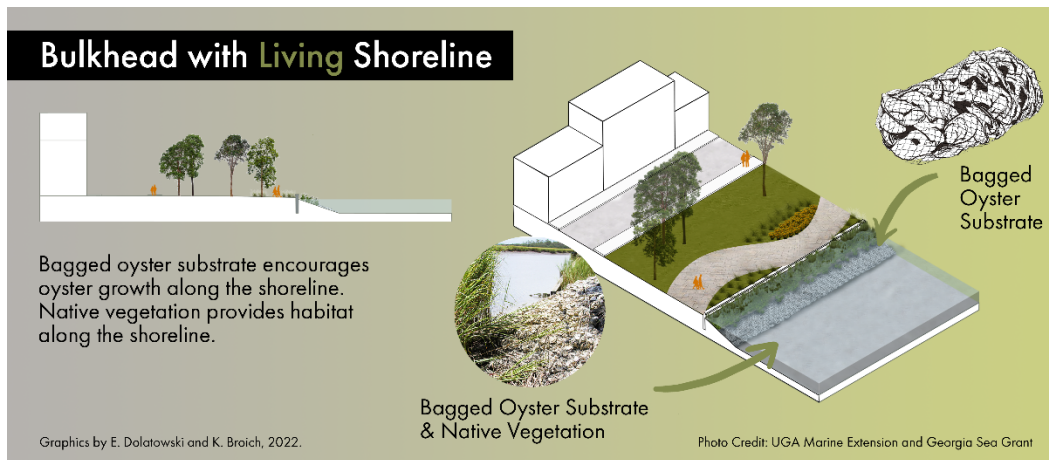
Figure 6. Rendering of a living shoreline feature combined with a conventional bulkhead to create hybrid infrastructure that enhances biodiversity value in a coastal environment.
