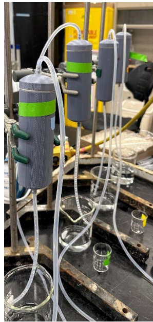
Figure 5. The 3D-printed cylinders in a vertical position for the ammonia removal experiments.
