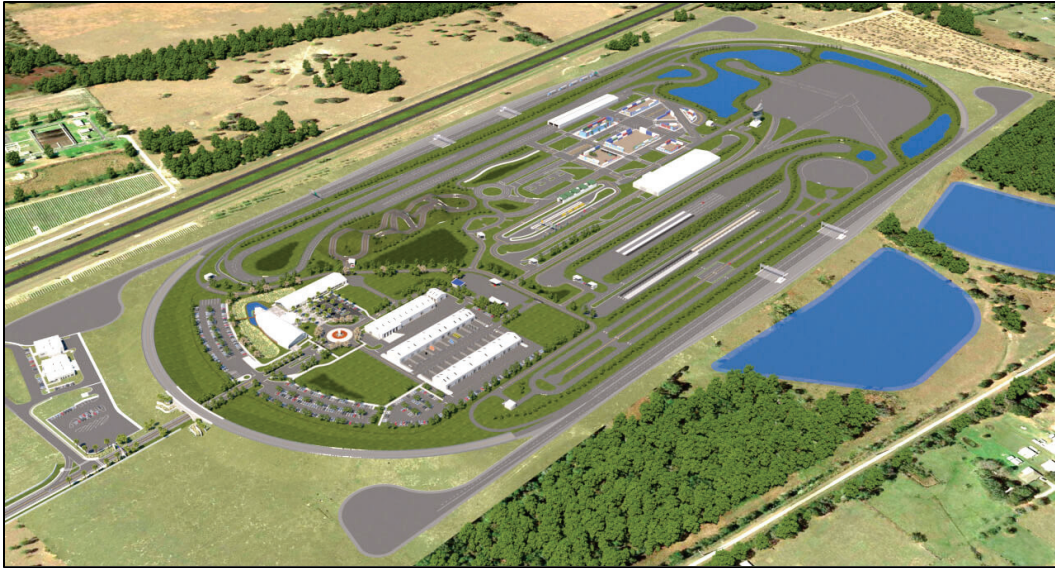
Figure 47. The SunTrax site features a large testing loop with connected infield testing areas and associated research facilities. (Image reproduced from Florida Department of Transportation, n.d. Public domain.)
