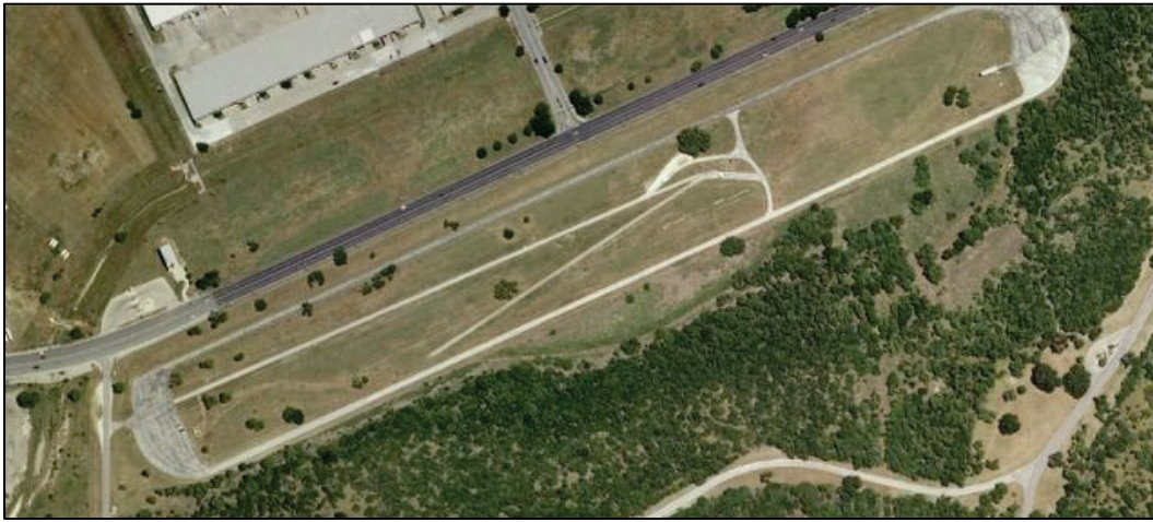
Figure 46. Satellite imagery of Southwest Research Institute (SwRI) features a 1.2 mi track loop to test transportation technologies. (Map data: Google Earth, n.d.)
