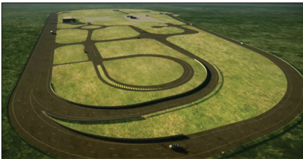
Figure 39. The PennSTART site features one large track loop with connected infield test environments and a technology laboratory. (Image reproduced with permission from the Commonwealth of Pennsylvania Department of Transportation 2019. Public domain.)
