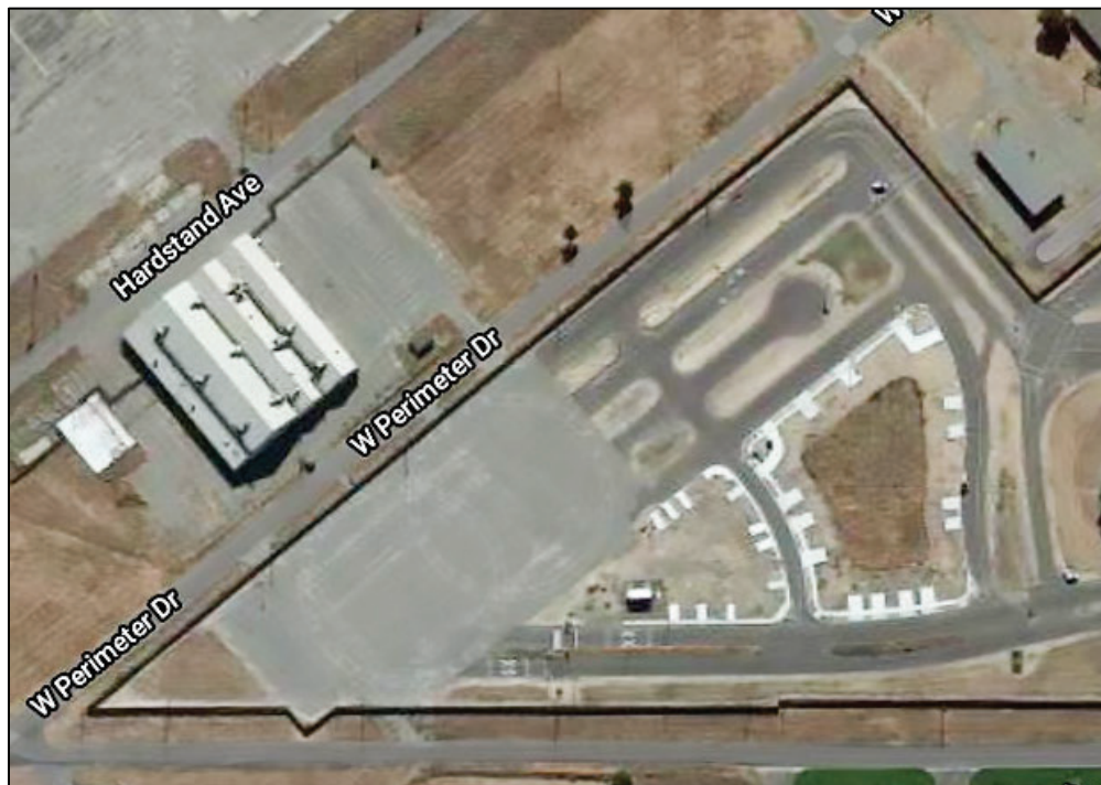
Figure 5. The Castle course showing that Castle makes use of existing roadways, marked open pavement ( left ), and newly poured concrete driveways and curbs ( right ) to test AVs. (Map data: Google Earth 2013.)
