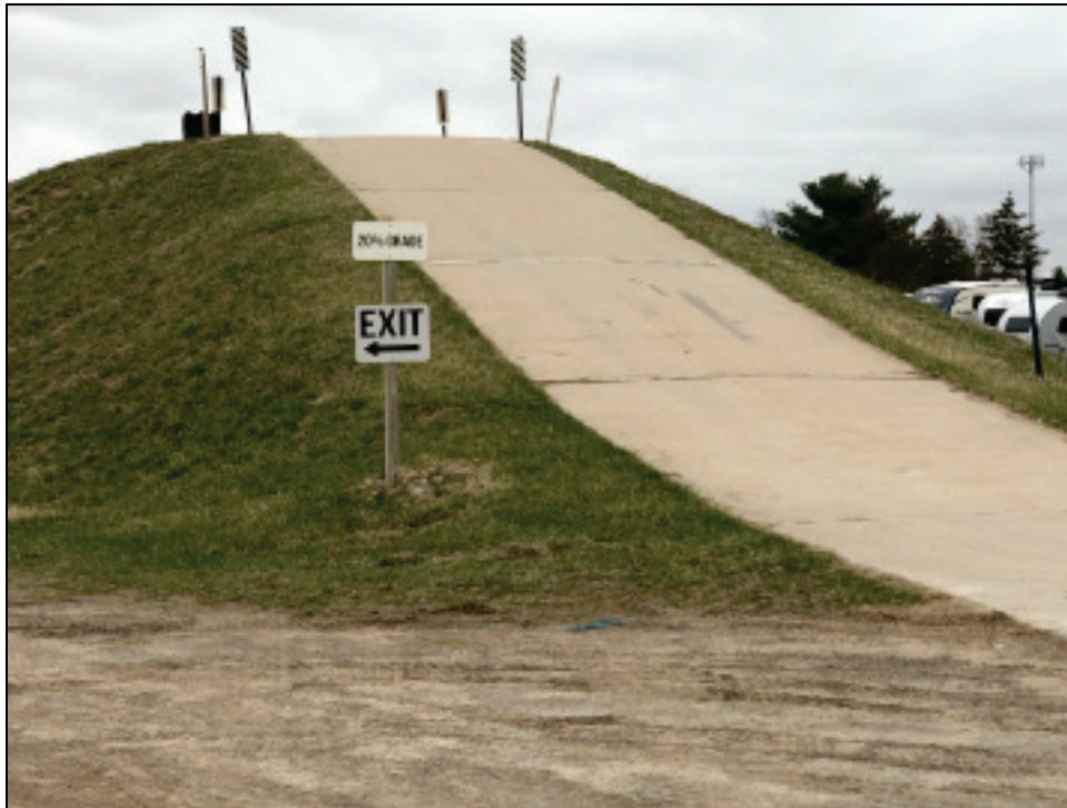
Figure 32. Vehicles at MITRP have access to a series of road simulations, including hill grades to test braking and stability. (Image provided by MITRP and used with permission.)
