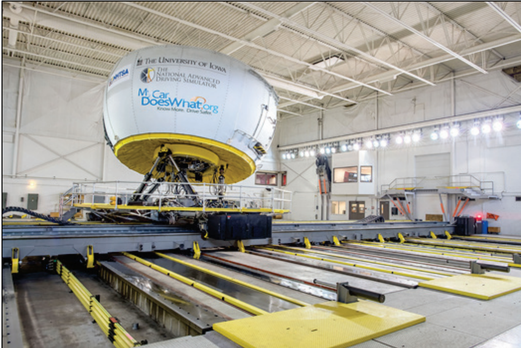
Figure 33. National Advanced Driving Simulator (NADS)-1 is a high-fidelity ground vehicle simulator with the largest motion range of any driving simulator in the United States. (Image reproduced with permission from University of Iowa, “National Advanced,” n.d.)
