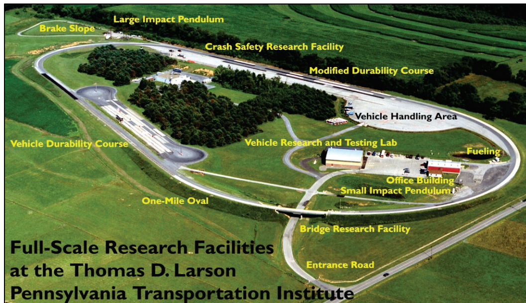
Figure 27. Research and testing facilities for the test track at Larson Transportation Institute (LTI) were developed to challenge vehicle handling in a variety of on-road conditions. (Image reproduced with permission from LTI, “Test Track,” n.d.)
