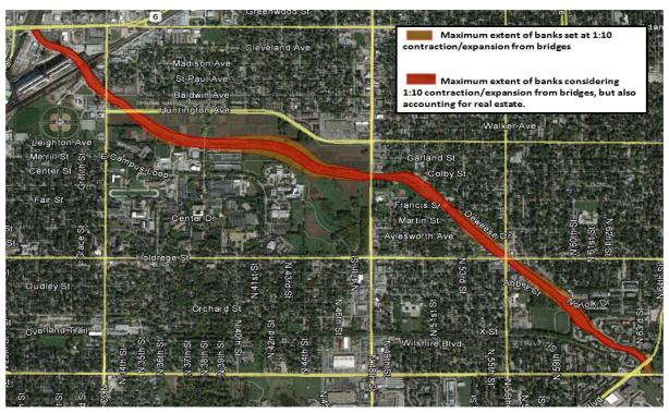
Figure 10. Contraction and Expansion at bridges being optimized to increase flow. Maximum channel extents vs realistic extents based on real estate.
