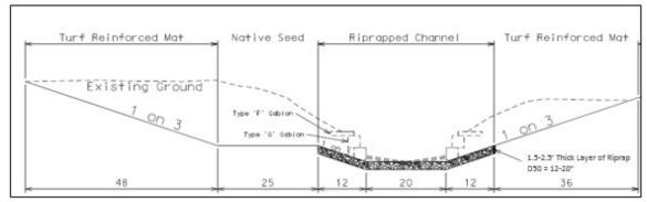
Figure 20. Comparison of the Existing vs. Proposed Channel Cross-Sections
