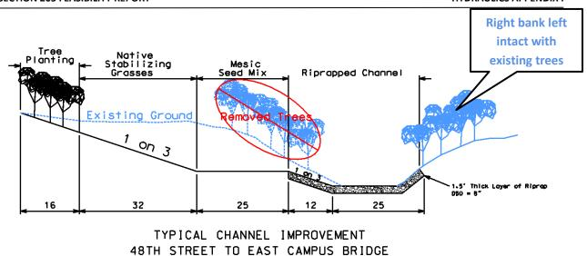
Figure 19. Proposed vs existing channel condition through Reach 2 (48th St Bridge to East Campus Bridge)
