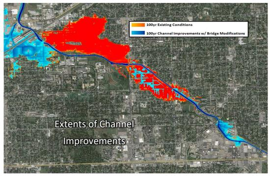
Figure 14. Channel Improvements with Bridge Modifications (7 bridges replaced, see Figure 15) versus Existing Conditions (Reach 2 and 3)
