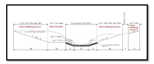
Figure 3. Typical cross-section of channel widening configuration from Cornhusker Avenue upstream to just east of 48th Street.
