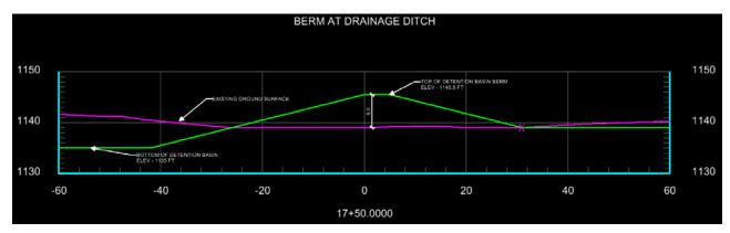
Figure 15. Detention Basin Embankment at Drainage Ditch.
