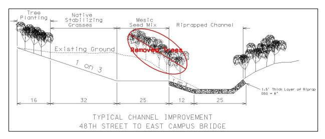
Figure 1. Typical cross section through East Campus, note the tree plantings on the upper banks of the channel footprint on the south bank, native stabilizing grasses placed on the reinforced turf mat, the mesic seed mix immediately adjacent to the channel and the undisturbed trees on the north bank
