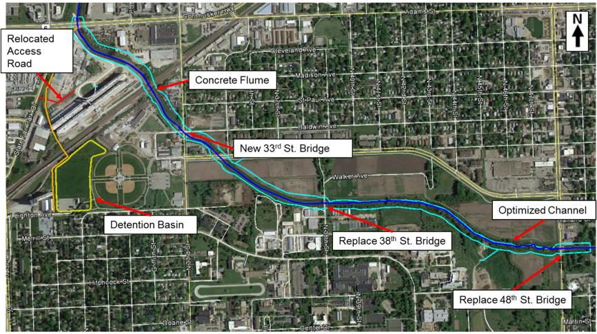
Figure 26. Optimized Recommended Plan
