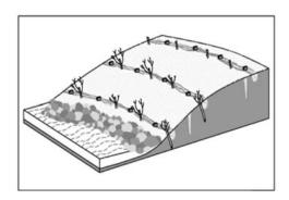
Live fascines are bundles of live (and nonliving) branch cuttings placed in long rows in shallow trenches across the slope on contour or at an angle. Fascines are intended to grow vegetatively while the terraces formed will trap sediment and detritus, promoting vegetative establishment. Fascines can be utilized as a resistive measure at the stream edge and for erosion control on long bank slopes above annual high water. Fascines are also an effective way to anchor ECBs and TRMs.
