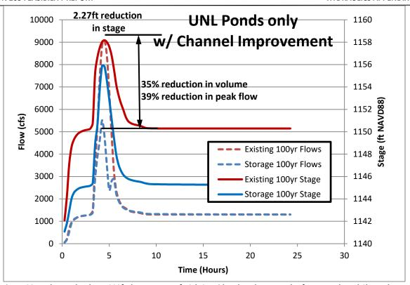
Figure 33. Hydrograph taken 1000ft downstream of 48th St Bridge that shows result of UNL Ponds and Channel Improvements
