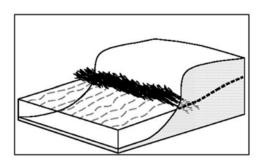
Live siltation is a bioengineering technique involving the installation of a living or a nonliving brushy system at the water's edge. Willow cuttings are the most common materials used. Live siltation construction is intended to increase roughness at the stream edge thereby encouraging deposition and reducing bank erosion. The embedded branches and roots also reinforce the bank and reduce geotechnical failure, while the branches and leaves provide cover, aquatic food sources, and organic matter.
