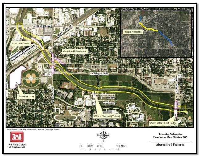
Figure 3. Components of the recommended plan.
