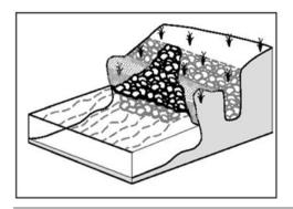
Trench fill revetments are constructed by excavating a trench along the top of the bank and placing stone riprap in the trench. As the bank erodes, the stone is undercut and "launches" down the bank line, resulting in a more gradual, protected slope. Earth removed for excavation of the trench may be used to cover the riprap, thus completely concealing it until it is launched. This technique might be chosen if access to the stream reach is restricted due to legal or environmental issues.
