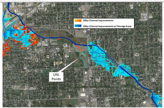
Figure 35. Flooding reduced at 33rd and 36th St bridges downstream of UNL ponds (w/ channel improvements and w/o Holdrege ponds).
