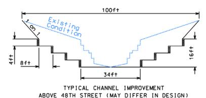
Figure 18. Proposed vs existing channel condition through Reach 3
