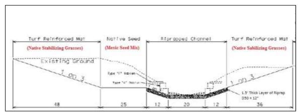
Figure 28. Typical Cross Section of Mitigating Actions along the Impacted Channel Footprint of Deadmans Run
