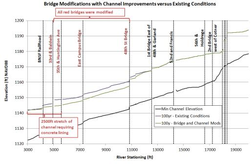
Figure 17. Bridge and Channel Improvements through Reach 2 only 100yr profiles
