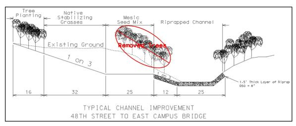
Figure 5. Typical cross section through East Campus, note the upper banks of the channel footprint on the south bank, native stabilizing grasses placed on the reinforced turf mat, the mesic seed mix immediately adjacent to the channel and the undisturbed trees on the north bank.
