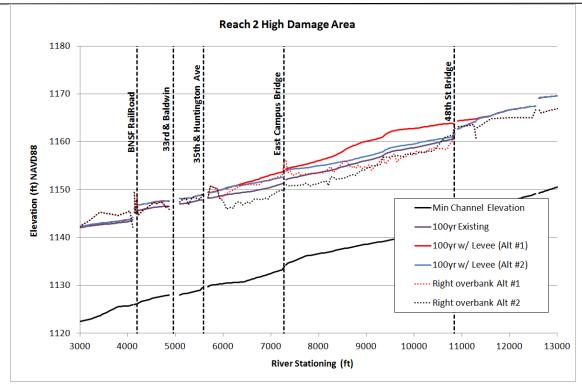
Figure 21. Water surface stage profile for Levee Alt #1 and #2 vs Existing Conditions
