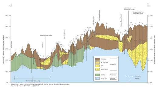
**Figure 5. Interpretive Geologic Cross Section B-B'**, North-South. The location of this cross section is shown on Figure 3. The dashed horizontal line is an estimated water level elevation and the solid vertical lines represent the locations of bore holes or registered well logs. Loess, till, silt, and clay deposits are not subdivided (Divine).
