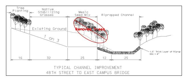
Figure 26. Typical cross section through East Campus, note the tree plantings on the upper banks of the channel footprint on the south bank, native stabilizing grasses placed on the reinforced turf mat, the mesic seed mix immediately adjacent to the channel and the undisturbed trees on the north bank.
