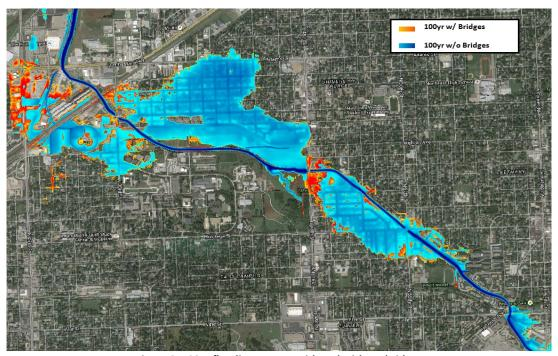
Figure 9. 100yr flooding extents with and without bridges
