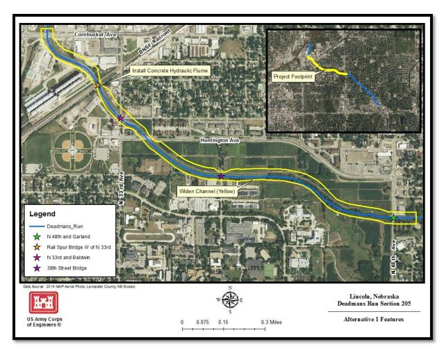
Figure 2. Proposed project components of the Preferred Alternative
