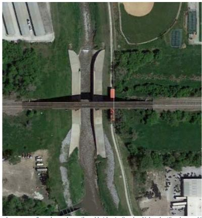
Figure 3. Example of a concrete flume beneath a railroad bridge in Omaha, Nebraska (Southeast of 84th Street and I-80)
