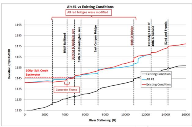
Figure 5. Alternative #1 vs Existing Conditions 100yr water surface profiles
