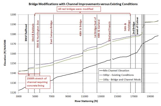
Figure 15. Bridge modifications and Channel Improvements vs Existing Conditions
