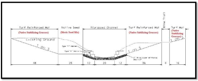
Figure 4. Typical cross-section of channel widening configuration from Cornhusker Avenue upstream to just east of 48<sup>th</sup> Street.
