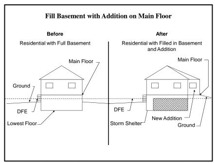
Figure 2: Schematic of Filled Basement with Main Floor Addition
