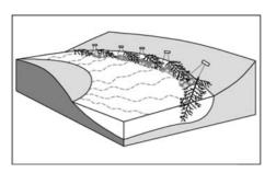
Rootwad revetments and tree revetments are structures constructed from interlocking tree materials. These structures are continuous and resistive, distinguishable from discontinuous and redirective techniques, such as LWD structures or rootwad deflectors. Rootwad revetments and tree revetments are primarily intended to resist erosive flows and are usually used on the outer bank of a meander bend when habitat diversity is desirable and tree materials are available and naturally occurring.
