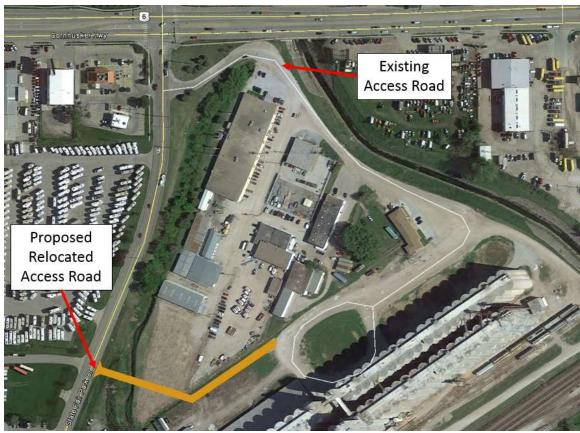
Figure 23. Existing & Proposed Relocated Access Road along the West Tributary
