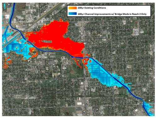
Figure 16. Bridge and Channel Improvements through Reach 2 only 100yr mapping
