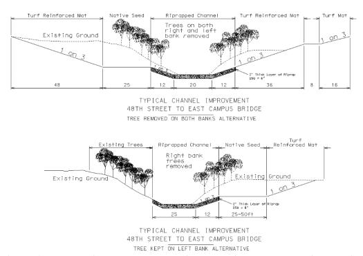
Figure 2. Typical cross section of Variation I (top image) and Variation II (bottom image) on Deadmans Run through East Campus.
