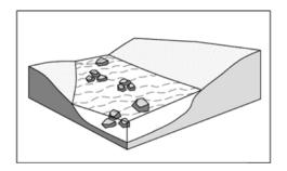
Large boulders may be placed in various patterned clusters within the base flow channel of a perennial stream. Natural streams with beds coarser than gravel often feature large roughness elements like boulders that provide hiding cover and velocity shelters for fish and other aquatic organisms. If a constructed or modified channel lacks such features, adding boulder clusters may be an effective and simple way to improve aquatic habitat.
