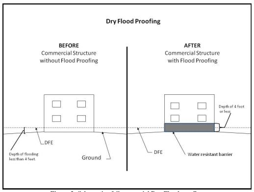
Figure 3: Schematic of Commercial Dry Floodproofing
