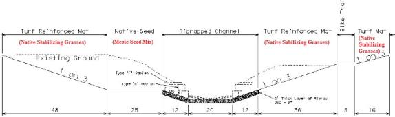
Figure 1. Typical cross section of proposed channel widening throughout Deadmans Run
