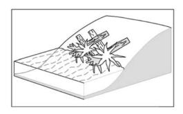
Large woody debris (LWD) structures (also known as engineered log jams) made from felled trees may be used to deflect erosive flows and promote sediment deposition at the base of eroding banks. Root wads, consisting of a short section of trunk and attached root bole, can also be used or incorporated into the structures. Using the classical spur design criteria and methods, the placement of LWD structures can be designed to achieve optimum benefit for both aquatic habitat and bank protection.
