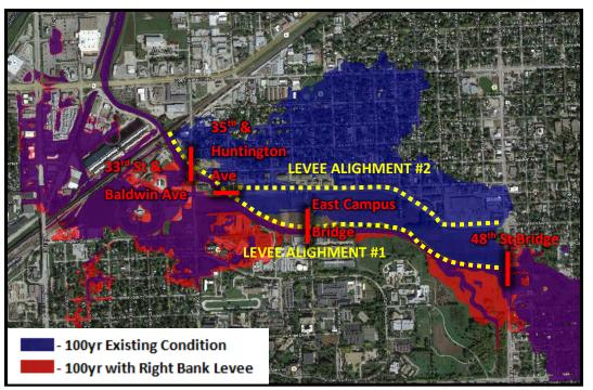
Figure 22. 100yr Existing vs Right Bank Levee
