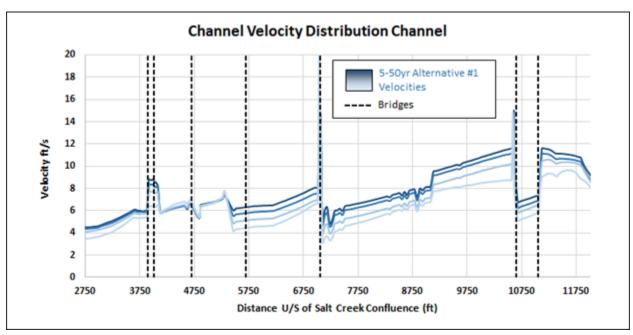
Figure 38. Velocity Distribution for Deadmans Run Channel Improvements
