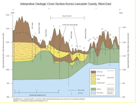
**Figure 4. Interpretive Geologic Cross Section A-A'**, West-East. The location of this cross section is shown on Figure 3. The dashed horizontal line is an estimated water level elevation and the solid vertical lines represent the locations of bore holes or registered well logs. Loess, till, silt, and clay deposits are not subdivided (Divine).
