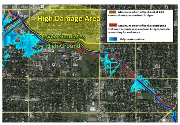
Figure 11. 100yr water surface added to channel only improvement analysis
