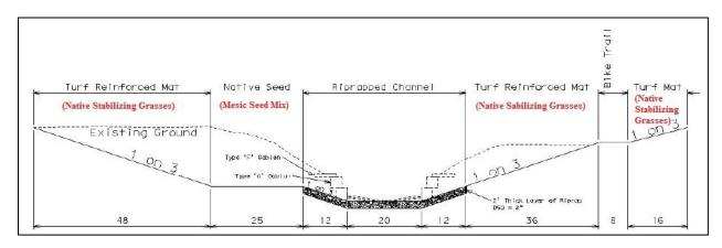
Figure 2. Typical cross section of mitigating actions along the impacted channel footprint of Deadmans Run, note the native stabilizing grasses placed on the reinforced turf mat and the mesic seed mix immediately adjacent to the channel.
