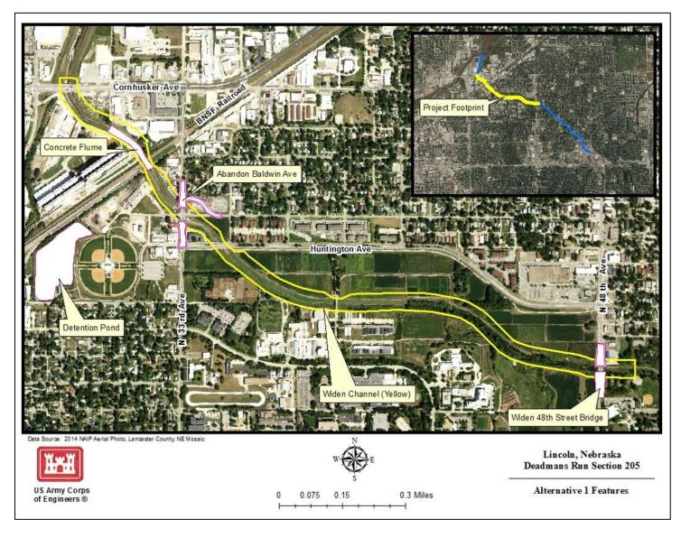
Figure 22. Structural features of Alternative 1 for Deadmans Run
