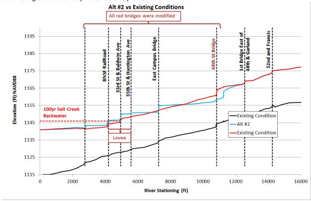
Figure 8. Alternative #2 vs Existing Conditions 100yr water surface profiles
