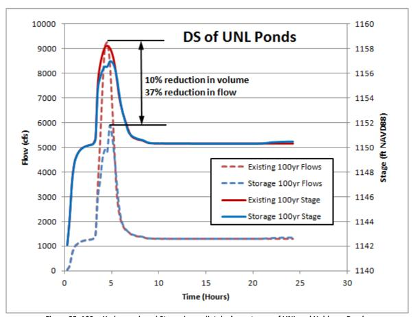
Figure 25. 100yr Hydrograph and Stages immediately downstream of UNL and Holdrege Ponds (HEC-RAS run includes both Holdrege and UNL ponds).
