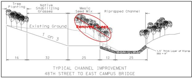
Figure 2. Typical cross section of Deadmans Run through East Campus.
