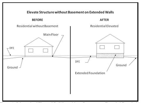
Figure 1: Schematic of Elevated Building without Basement on Extended Foundation
