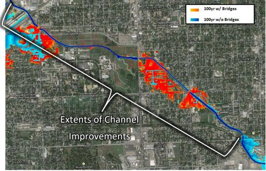
Figure 13. Channel Improvements with Bridge Modifications, all bridges removed.
