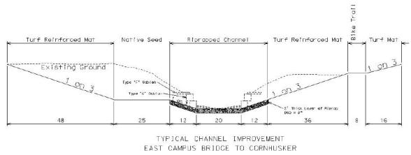
Figure 21. Typical cross section of proposed widening and improvement along Deadmans Run from Cornhusker Highway upstream to  $48^{\rm th}$  Street.
