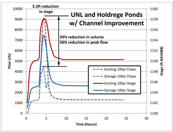
Figure 31. Reduction in Stage and Flow downstream of UNL ponds due to Storage at UNL and Holdrege w/ Channel Improvements
