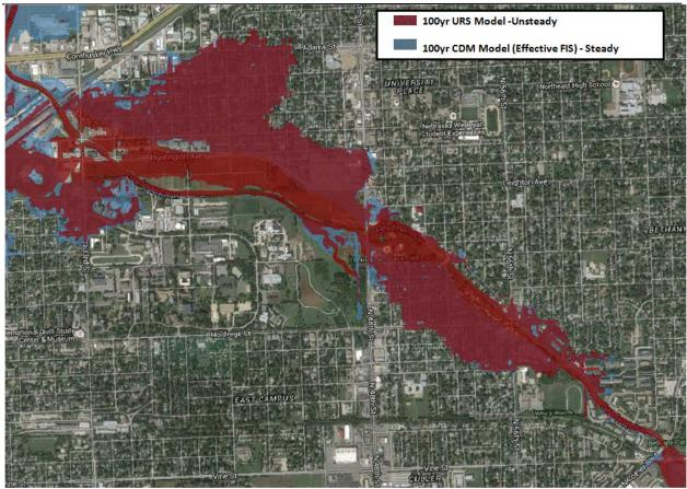
Figure 3. Existing FIS vs Unsteady Model 100yr Flooding Extents
