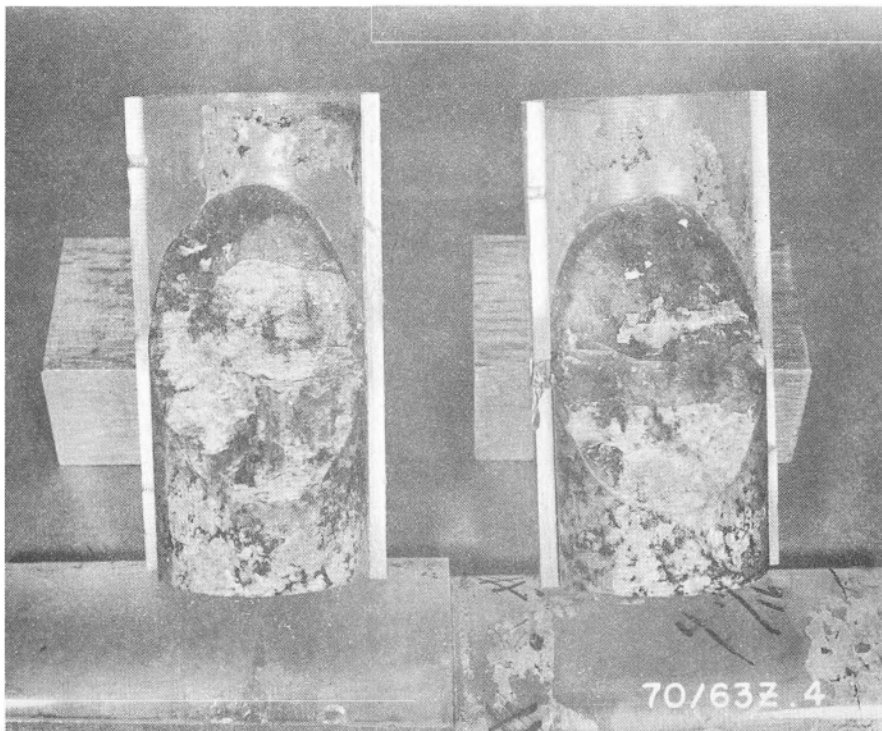
(a) Sawed halves of lucite tubing to remove bonded cores. Also shows Core No. 12 bonded with polyester resin which separated during sawing.
