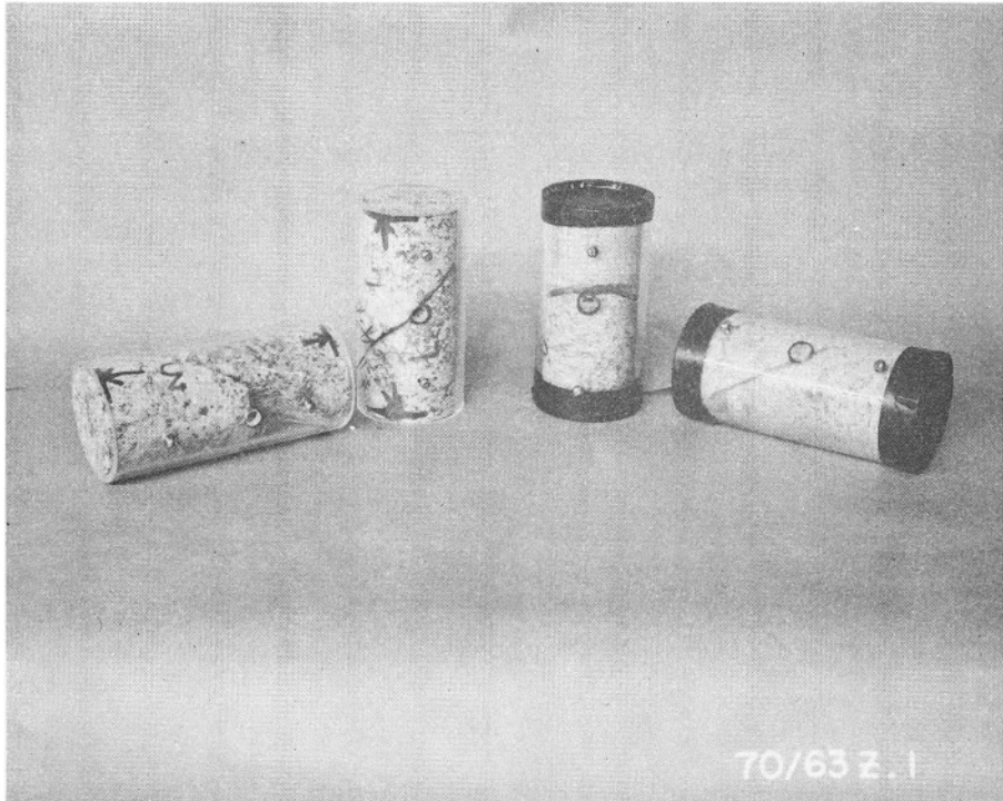
(a) Alignment and spacing of rock cores in lucite tubing, and showing end closure by neoprene tape to prevent leakage of grout.
