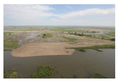
Figure 3. Levee breach closure and landward scour holes/sand dunes at L-575 "B" inlet breach (Sept. 2019)
