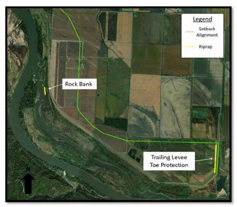
Figure 13. Plan view of riprap locations for setback alternative and rock bank location
