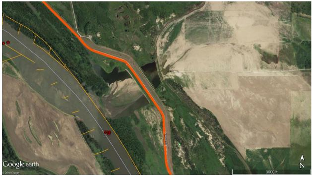
Figure 4. Small-scale levee setback along the Missouri River levee system L-550, near Watson, MO, river mile 539. Some landward and riverward scour holes remained following closure of this levee breach in 2012.
