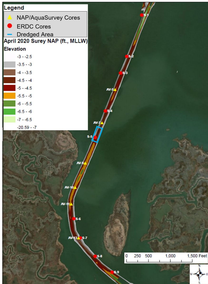
Figure 10. Seven Mile Island Innovation Laboratory (SMILL) – Intercoastal Waterway bathymetry and sample locations.
