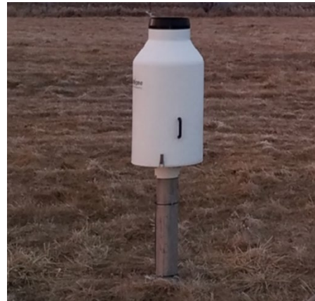
Figure 4. Weighing precipitation gauge, without a shield. Photo derived from Edwards & Behnke, 2019.
