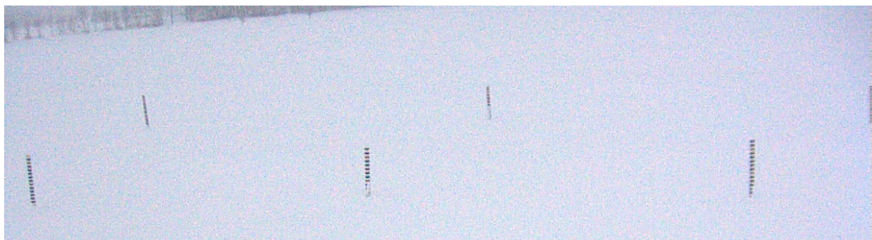
Figure 9. Snow stake field as viewed by Campbell CCFC camera (cropped images). Stakes use 1-inch black bands with 1-inch spacing.
