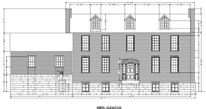
Figure 10. Jenkins House, north elevation. Example of measured elevation drawing to document and record original materials, scale, proportions, and features for restoration efforts when needed. (Huntington District, U.S. Army Corps of Engineers, August 2007)
