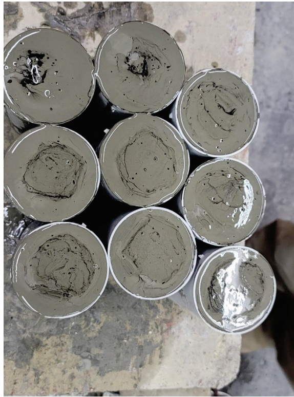
Figure 8. 0.3% (w/w) graphene in CGG-cement mixtures in plastic cylinders.
