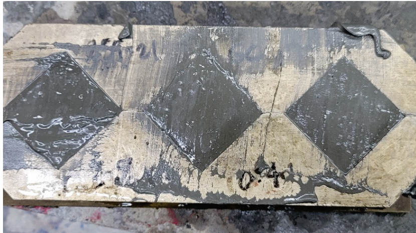
Figure 7. 0.3% weight for weight (w/w) graphene in commercial-grade graphene (CGG)-cement mixtures in steel mold.
