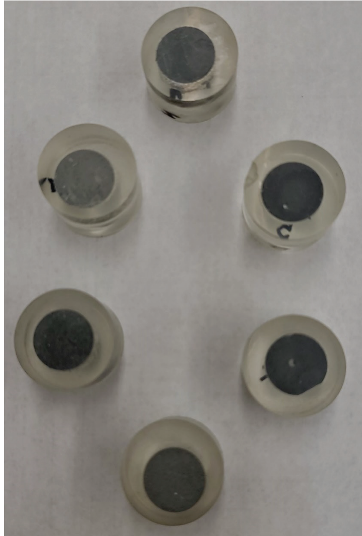
Figure 27. Polished graphene-cement samples for SEM/EDS.
