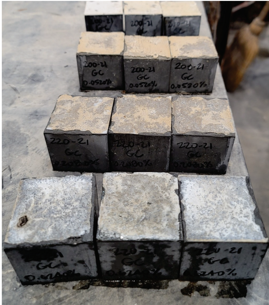
Figure 17. LGG-based cement cubes obtained with 0.02% (w/w) to 0.62% (w/w) graphene percentages.
