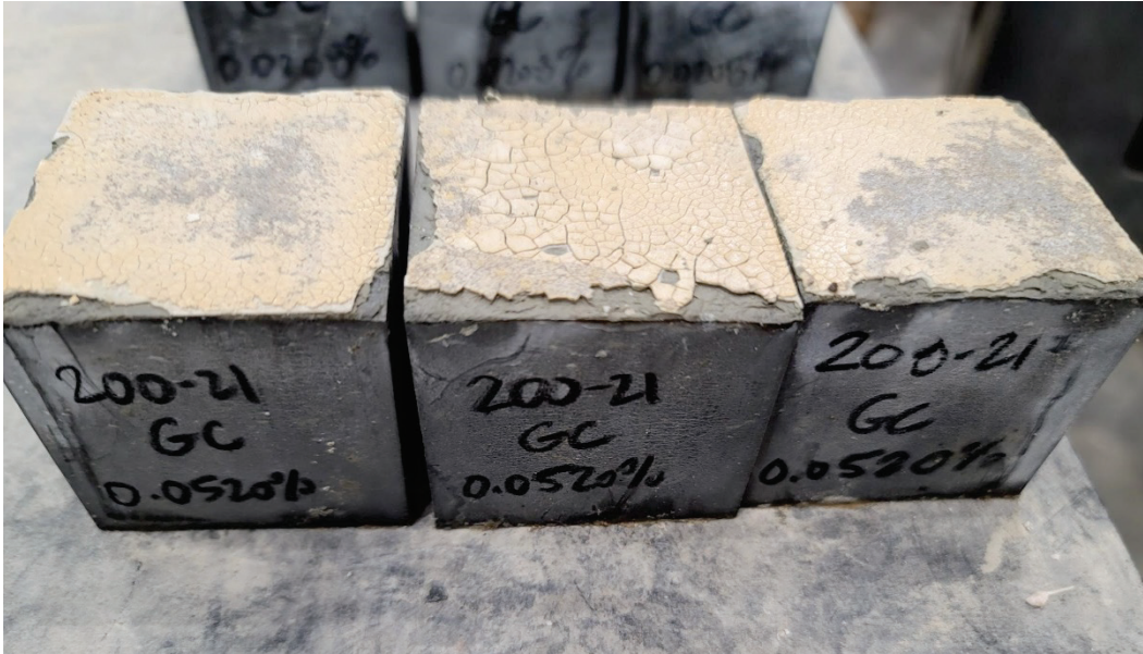
Figure 18. LGG-based cement cubes with 0.05% (w/w) graphene percentage.
