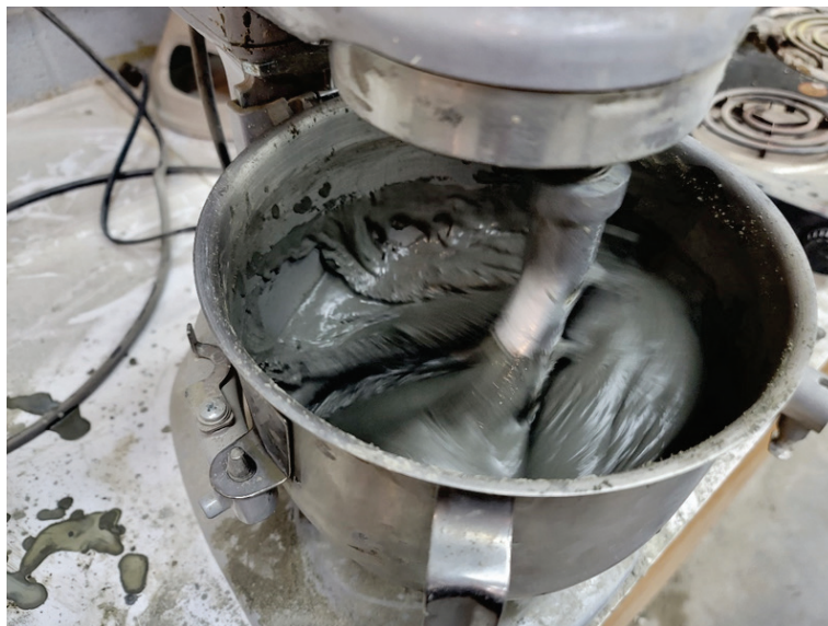
Figure 6. Graphene-cement mixture prepared in Hobart mixer bowl with dispersant.
