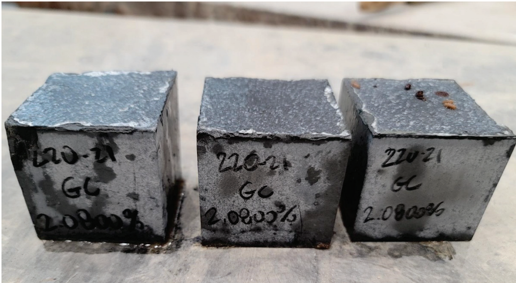
Figure 19. LGG-based cement cubes with 2.08% (w/w) graphene percentage.
