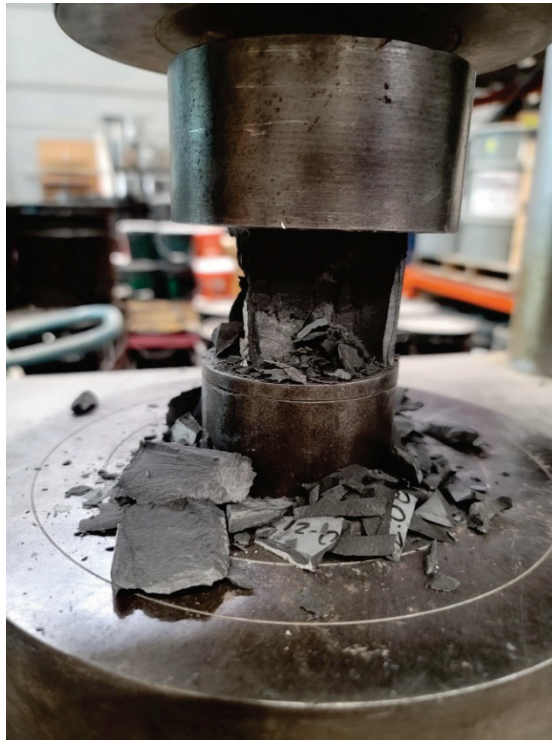
Figure 10. After the application of load to 0.02% (w/w) LGG-cement paste.
