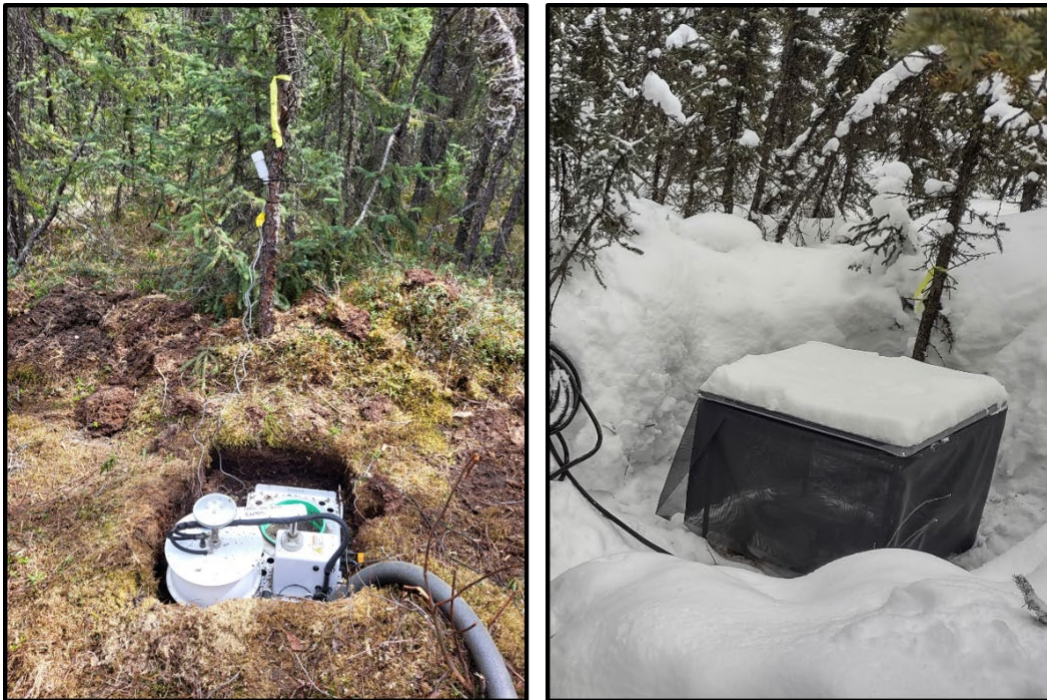
Figure 5. The 8100-104 long-term chamber deployed during warmer months ( right ) and the 8100-104 long-term chamber deployed during winter months with setup modifications to protect from heavy snowfall ( left ).
