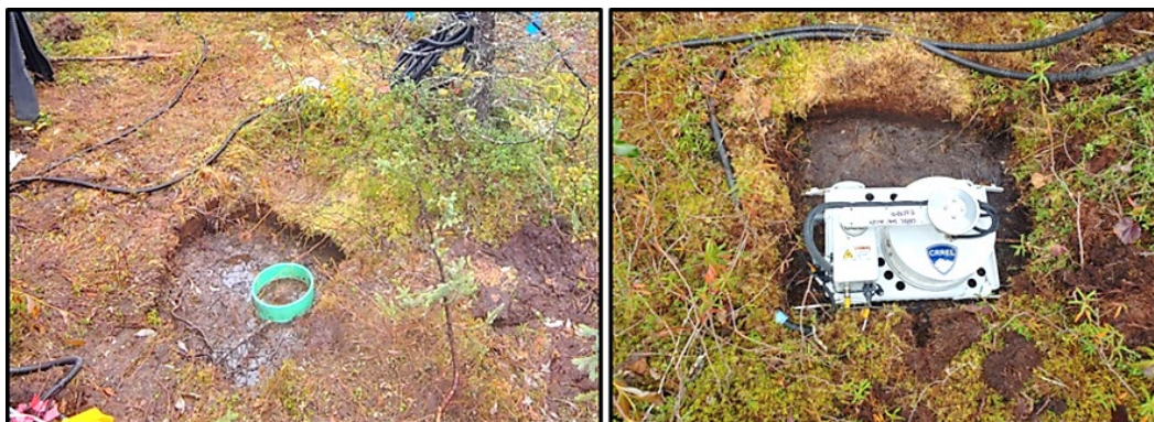
Figure 3. Image of vegetation removed from the chamber location with the soil collar visible ( left ) and chamber installed on the soil collar ( right ).
