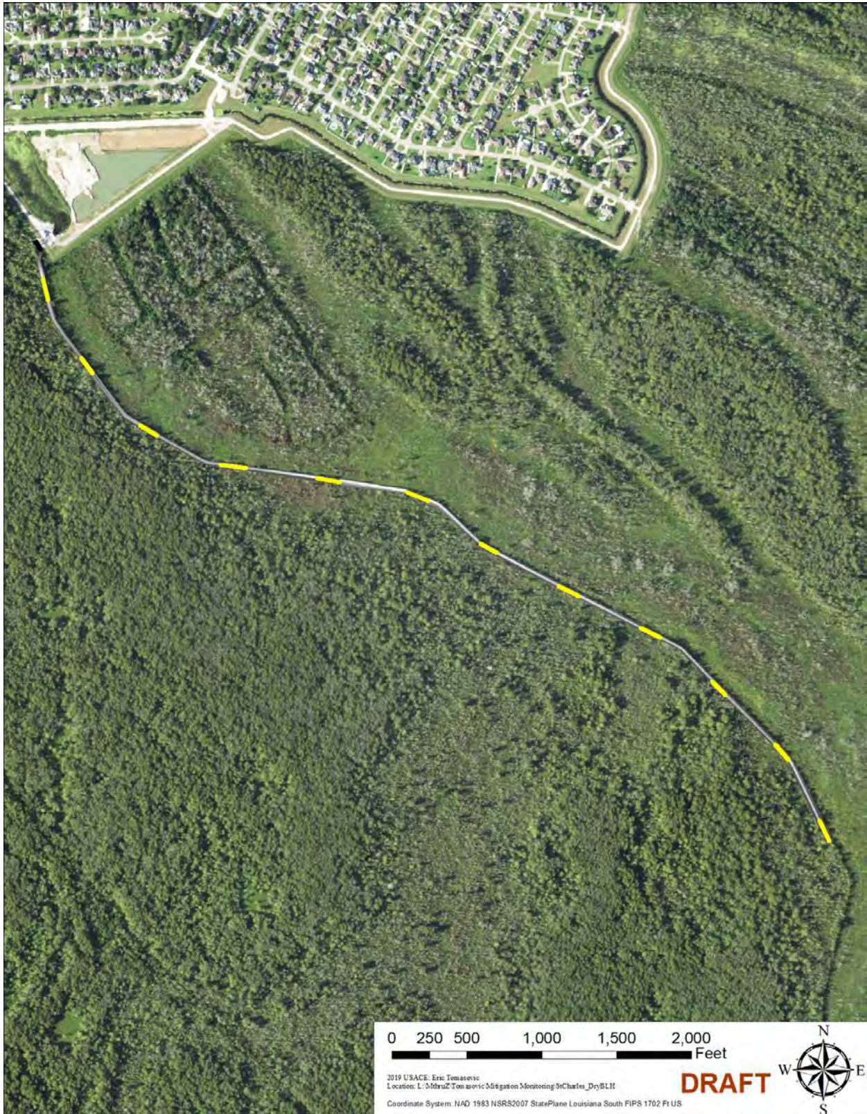
Figure 1. St. Charles BLH/swamp Mitigation berm cut locations to increase laminar flow.
