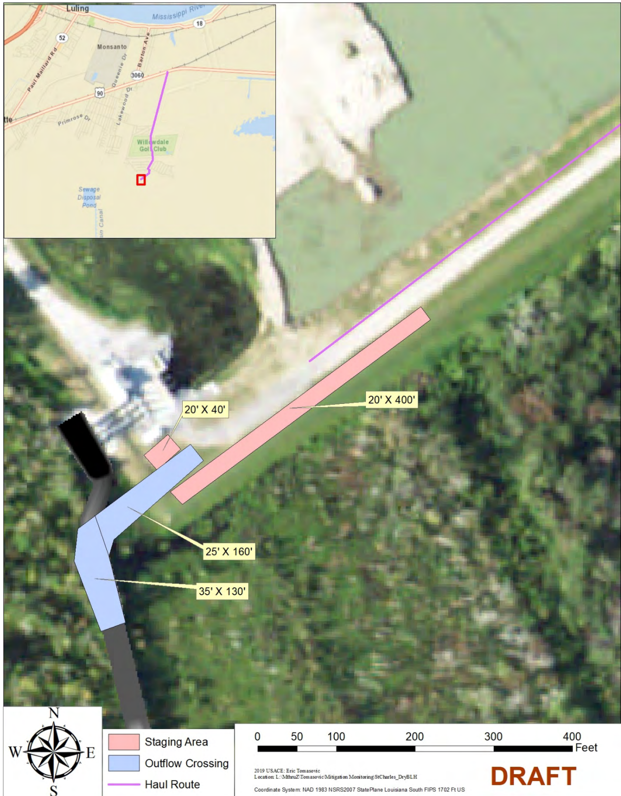
Figure 4. Staging area at the pump station, including outflow crossing.
