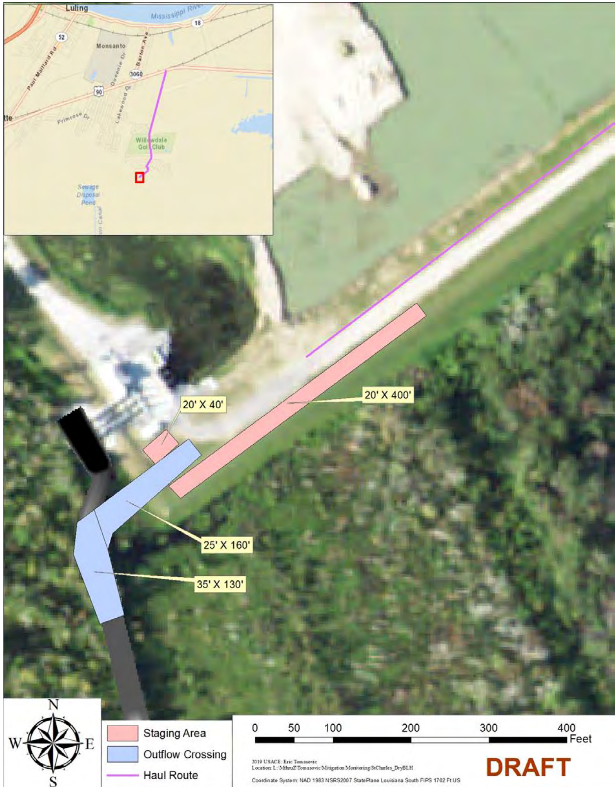
Figure 2. Staging area at the pump station, including outflow crossing.
