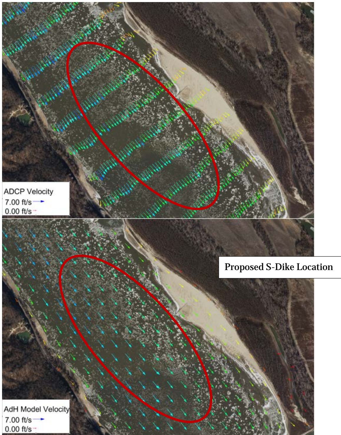
Figure 28. ADCP (top) compared to AdH Model Velocity (bottom) in the Proposed S-Dike Construction location.
