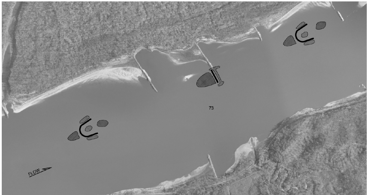
Figure 3 – Anticipated Deposition and Scour Patterns at Proposed Chevrons and Rootless Dike Extension MRM 72-74
