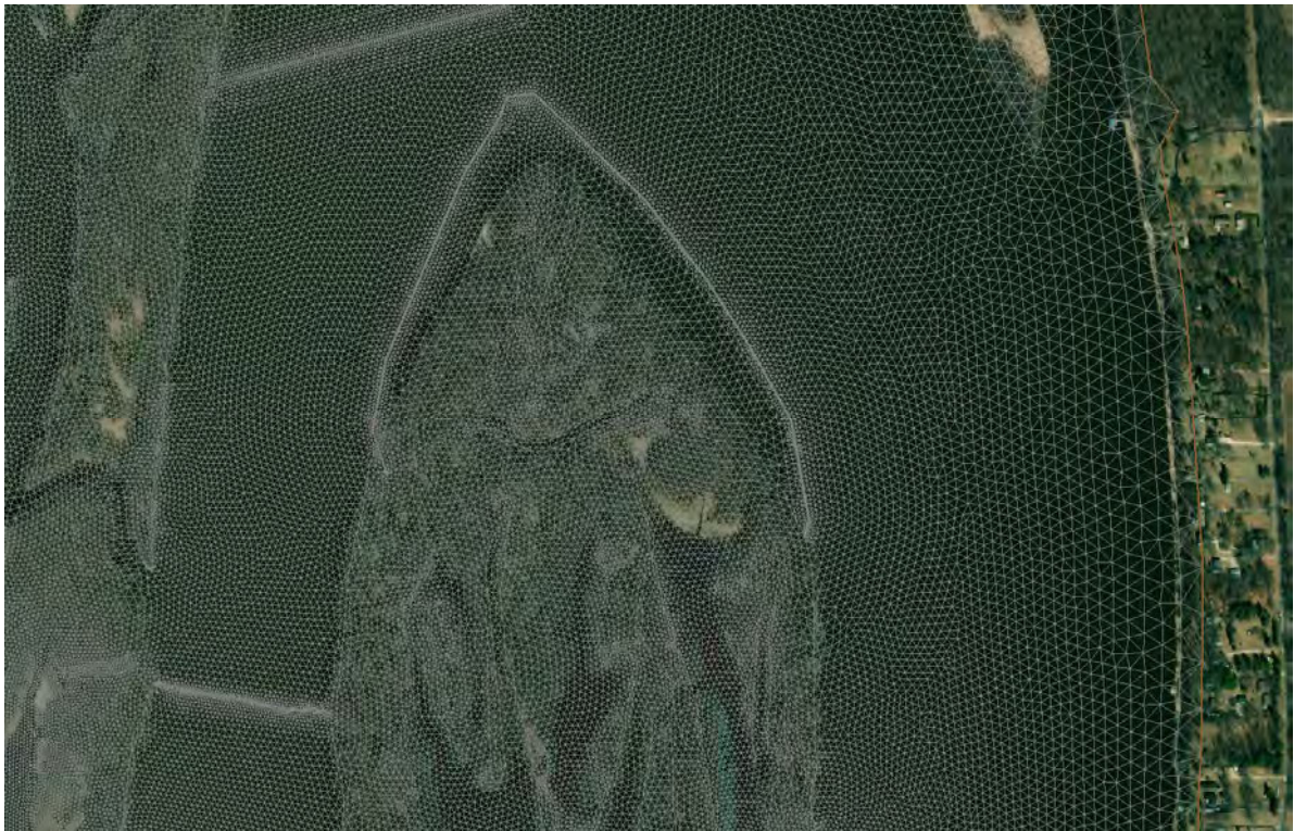
Figure H-12: AdH Model Mesh Depicting the Head of Steamboat Island
