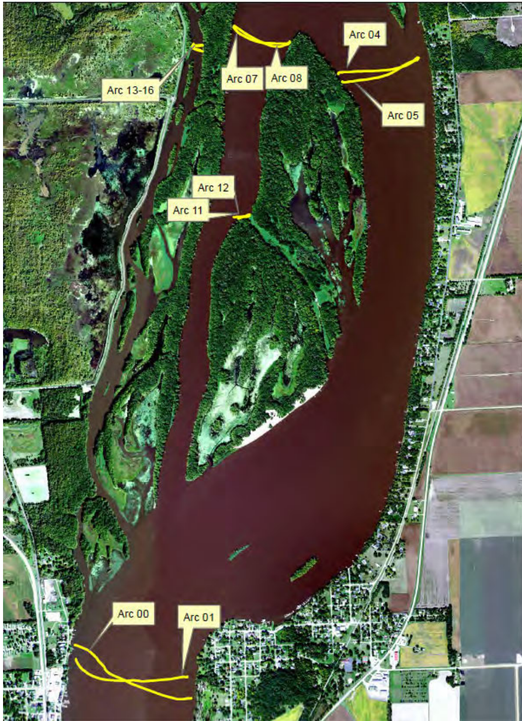
Figure H-13: July 2017 ADCP Transects at Steamboat Island
