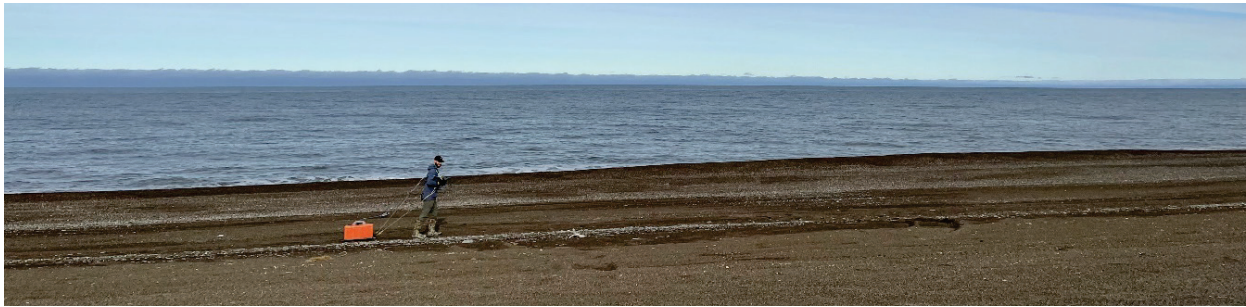
Figure 7. Project team member uses ground-penetrating radar (GPR) along the shoreline to assess permafrost and groundwater in the subsurface. (Photo credit: Lauren Bosche.)
