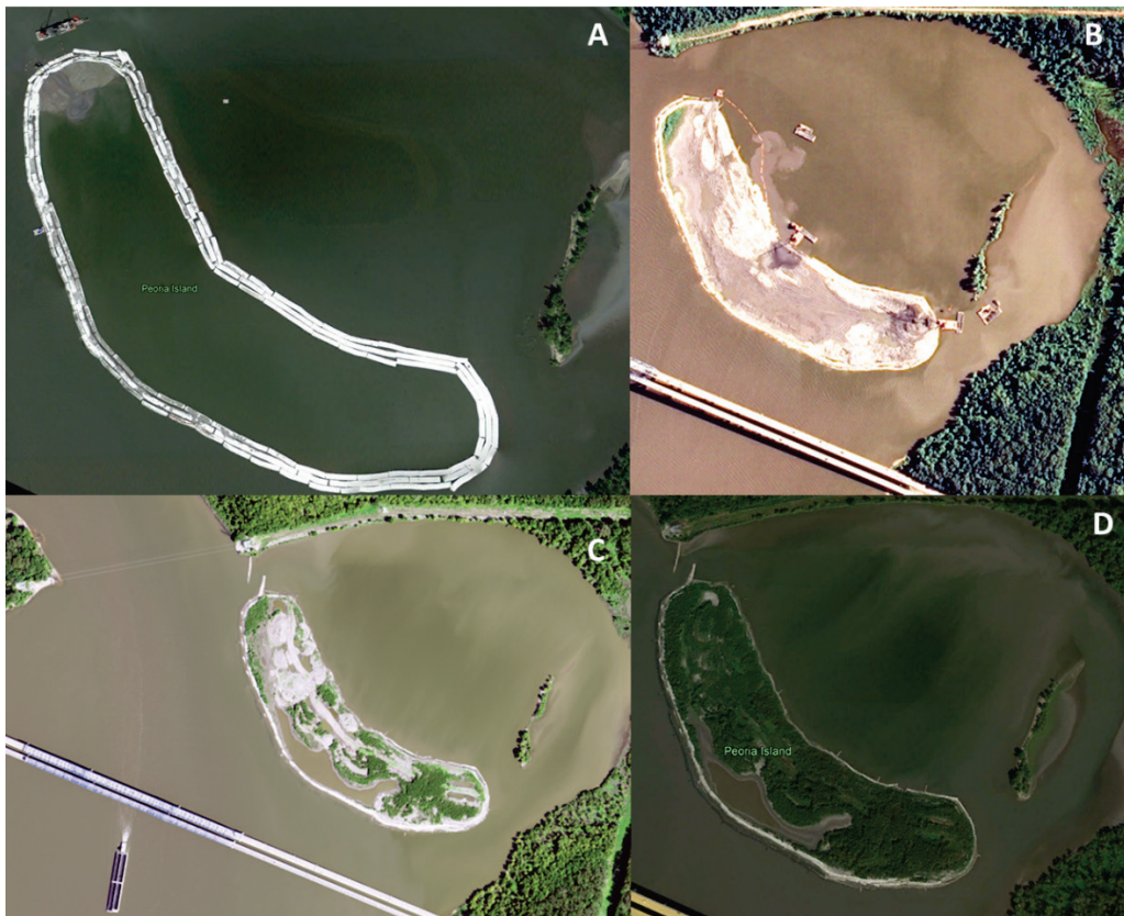
Figure 6. Stages of Peoria Riverfront Island, Illinois River. (A) Perimeter construction from filling of geotextile tubes in 2010, (B) interior construction in 2012, (C) island completion in 2015, and (D) increase in vegetation cover in 2017.
