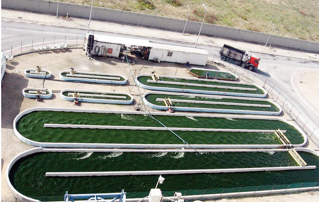
Figure 3. Multiple experimental raceway pond units show scaling options. (Photo courtesy of the US Department of Energy Renewable Energy Laboratory).
