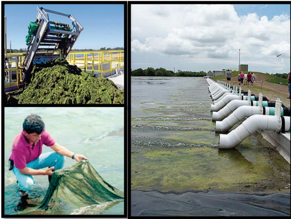
Figure 5. Large-scale algal turf scrubber demonstration in Ocala, FL (Source: Hydromentia, Ocala, FL).
