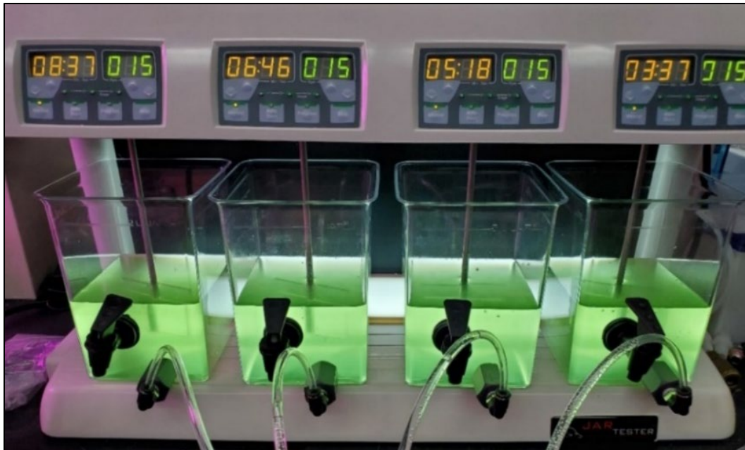
Figure 3. Four-station programmable, backlit Microfloc Platypus Jar Tester.
