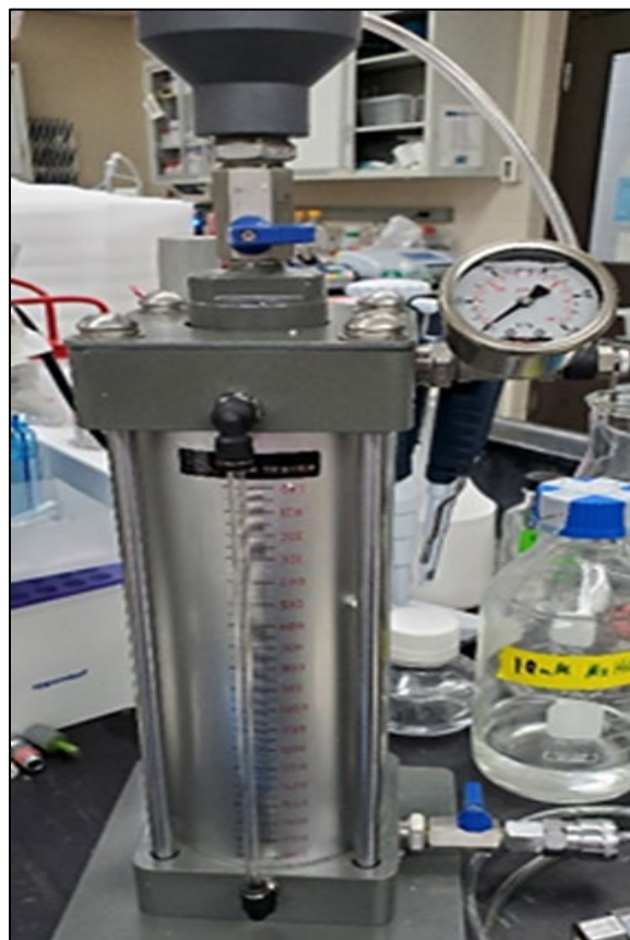
Figure 4. Microfloc dissolved air flotation (DAF) saturator assembly.
