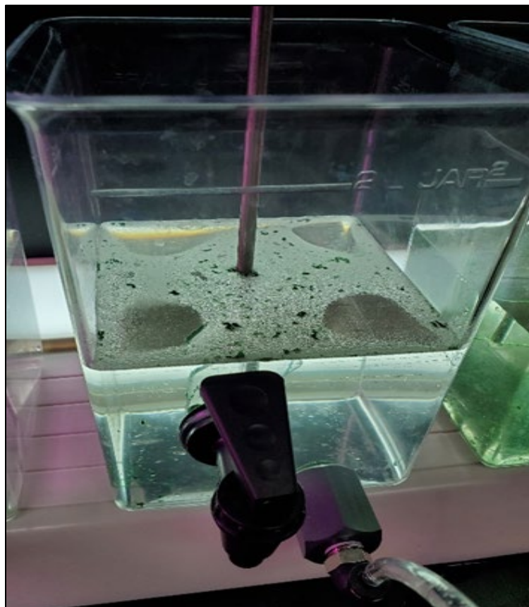
Figure 17. TF222 and XG after flocculation and flotation treatment.
