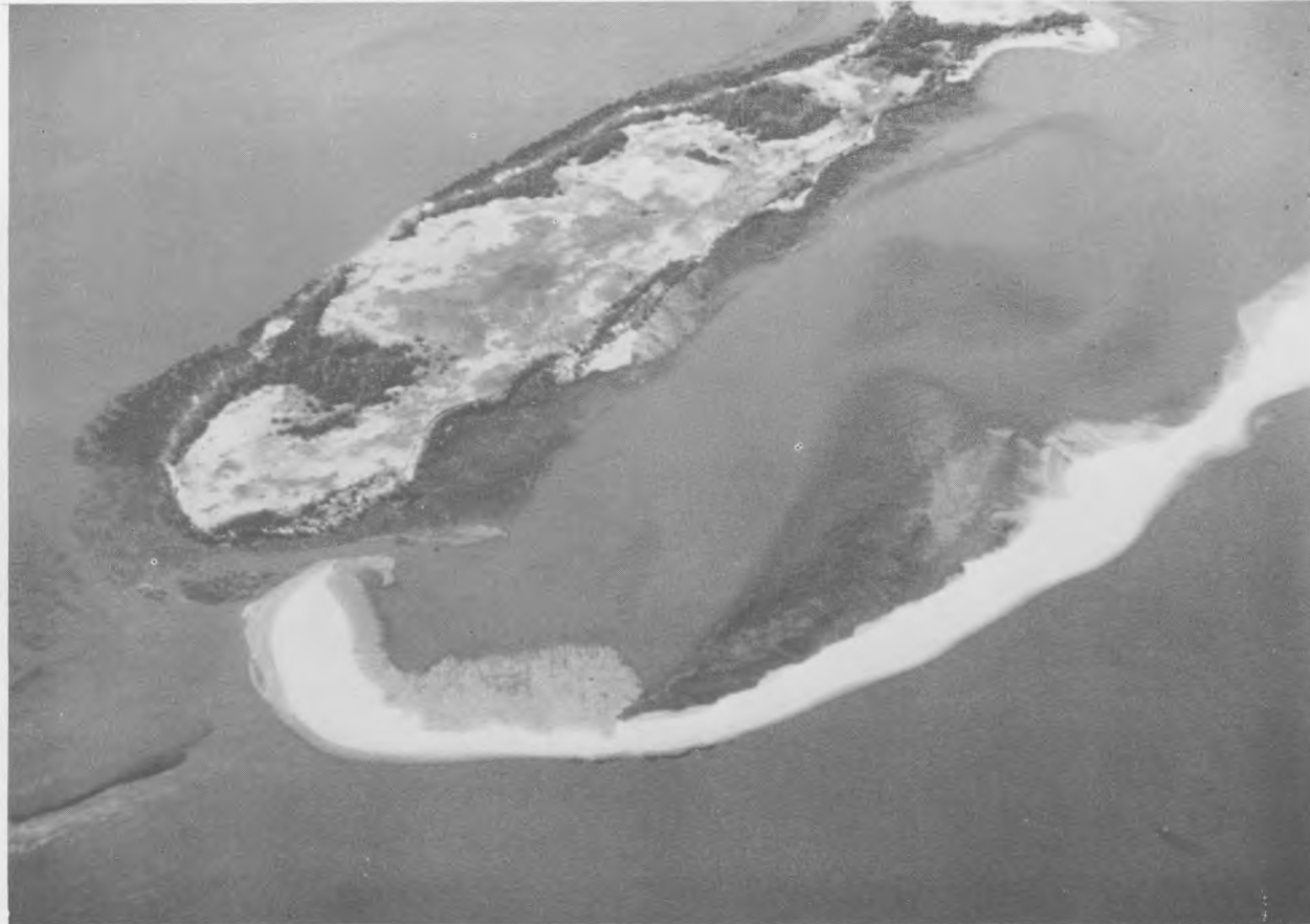
Figure 2. Aerial photograph of Miller Sands looking southwest with downstream being to the right. The marsh study plots are on the gray area just to the left of center in the foreground. Newly placed sand on the spit is clearly seen as the white areas. The lagoon and the older main island are also clearly evident
