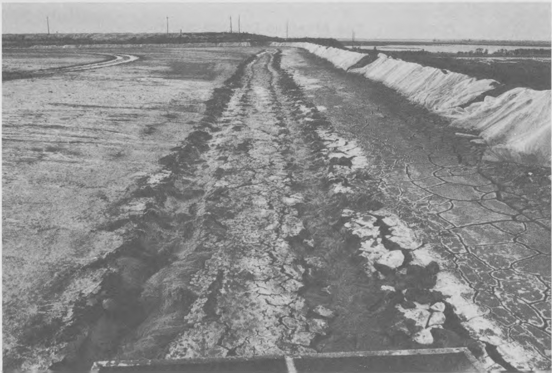
Figure 14. Twin ruts formed in disposal area surface crust by passage of the RUC
