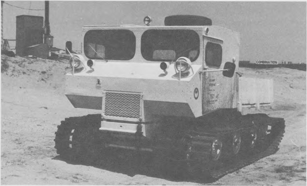
a. Thiokol Trackmaster with ground pressure of approximately 1.0 psi
