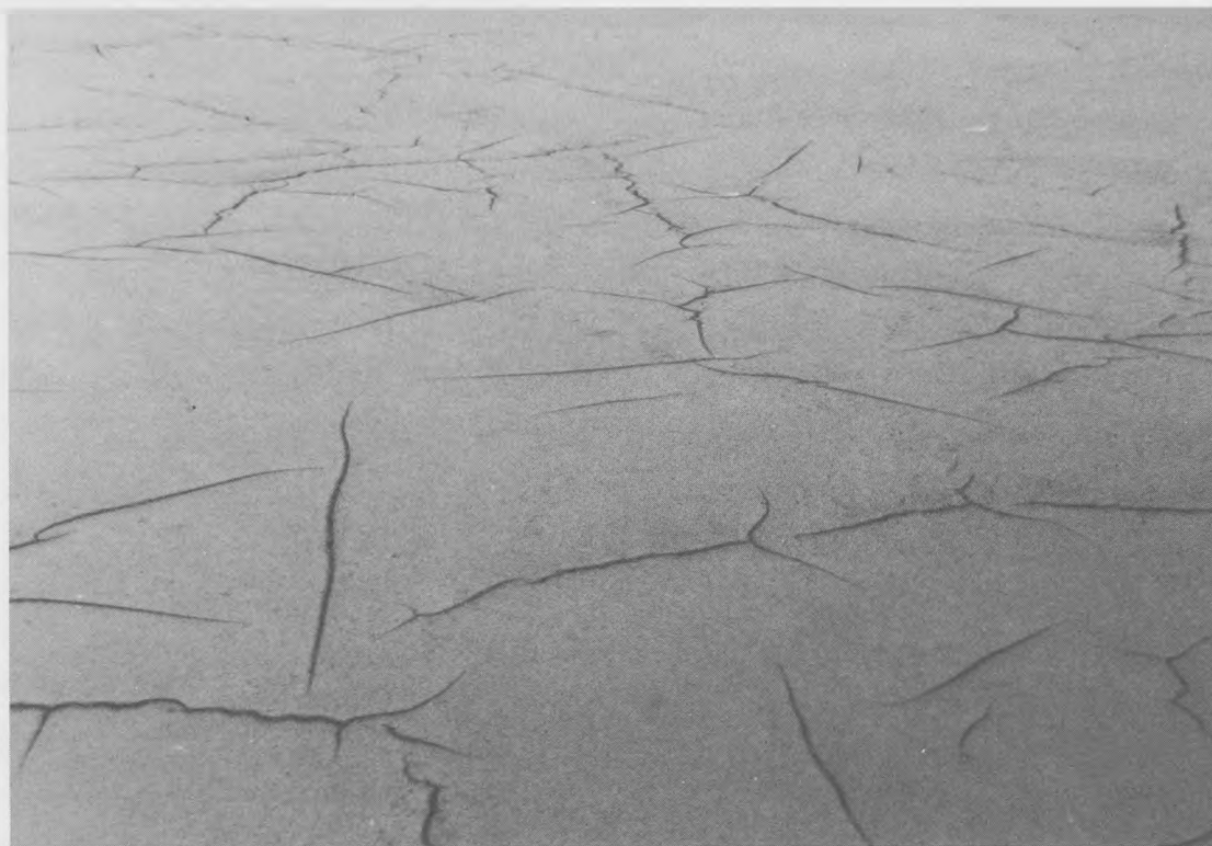
Figure 1. Surface of fine-grained dredged material at the earliest time when surface trenching should be attempted; initial cracks are spaced at 3- to 6-ft intervals and the surface water content approaches 1.8 \times LL
