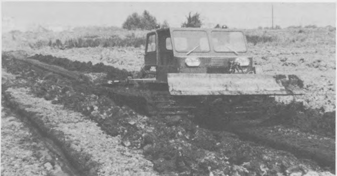
b. Wider-tracked Thiokol Spryte with ground pressure of approximately 0.6 psi
