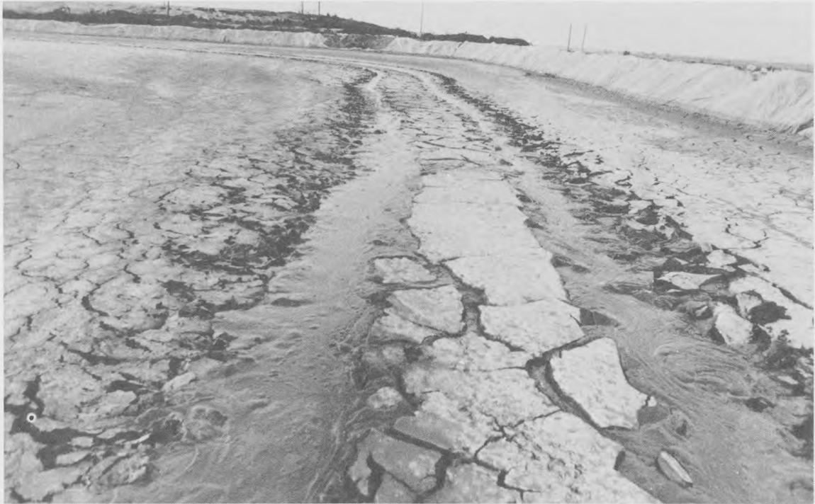
Figure 15. Twin shallow depressions created by the RUC in disposal area surface when a thin surface desiccation skin is present
