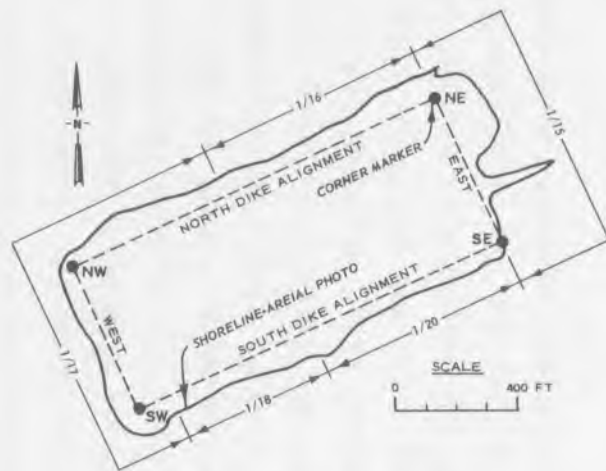
a. DRAGLINE FILL CONSTRUCTION SCHEDULE
