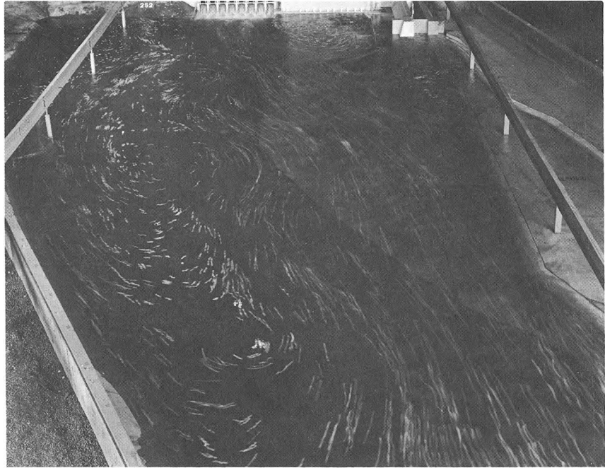
Photograph 21. Flow patterns in tailrace; final structures and excavation plan. River discharge 850,000 cfs, powerhouse closed.
