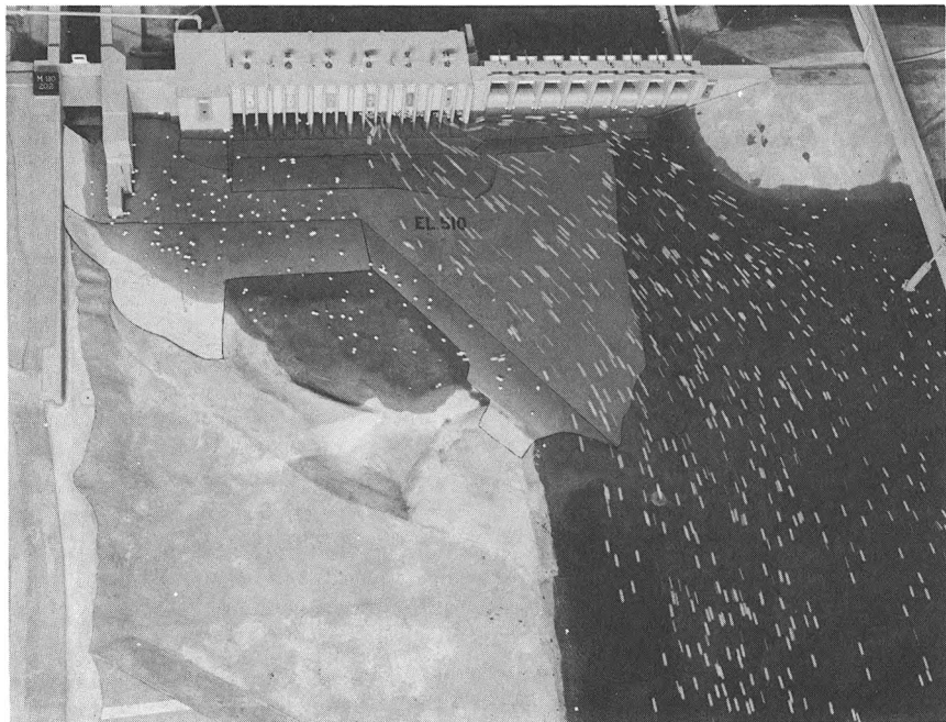
Flow patterns: river discharge 120,000 cfs
