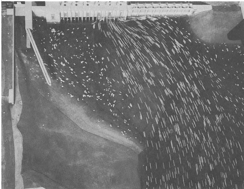
Flow patterns: river discharge 120,000 cfs
