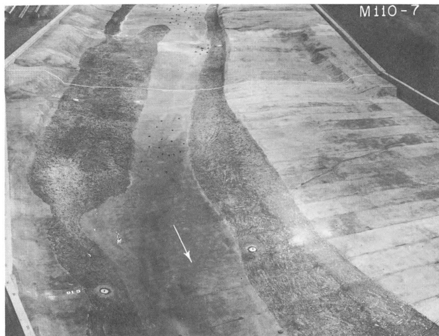
Fig. 2. Views of general model after verification of original river channel. The project axis is the white line across the model.
