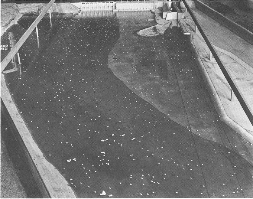
River discharge 25,000 cfs
