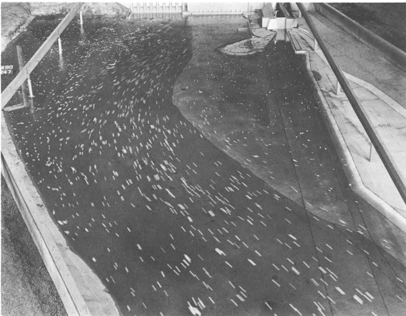
Powerhouse units 1 to 6 in operation
