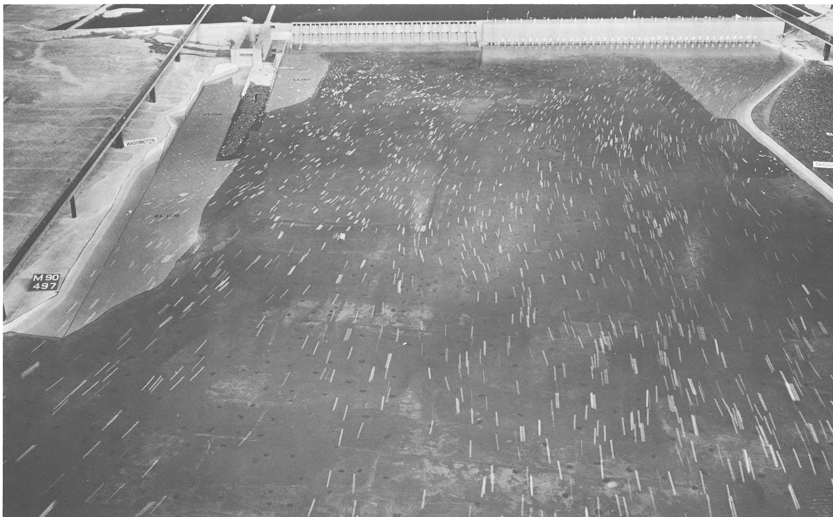
Photograph 29. Flow patterns downstream from final design structures; river discharge 600,000 cfs; powerhouse discharge 460,000 cfs, units 1 to 20; spillway discharge 137,075 cfs, uniformly distributed among bays 2 to 20, 2700 cfs through bay 1; fishway flow 225 cfs.
