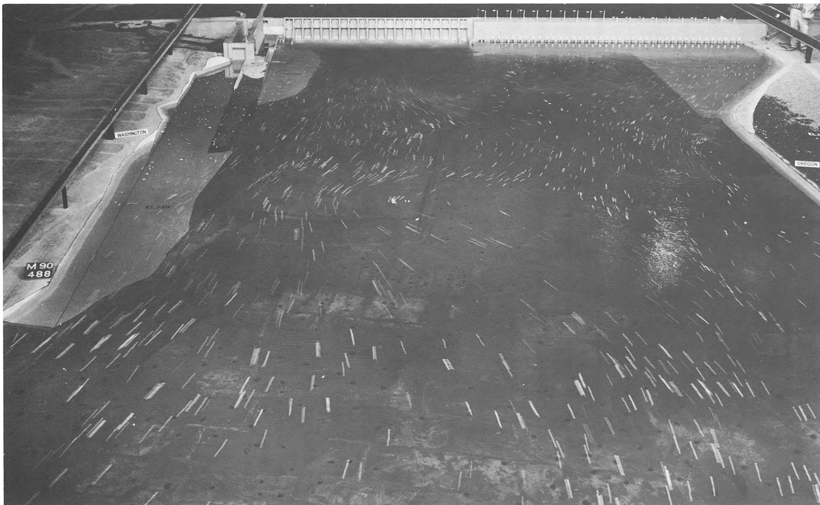
Photograph 28. Flow patterns downstream from final design structures; river discharge 600,000 cfs; powerhouse discharge 230,000 cfs, units 1 to 10; spillway discharge 367,075 cfs, uniformly distributed among bays 2 to 20, 2700 cfs through bay 1; fishway flow 225 cfs.
