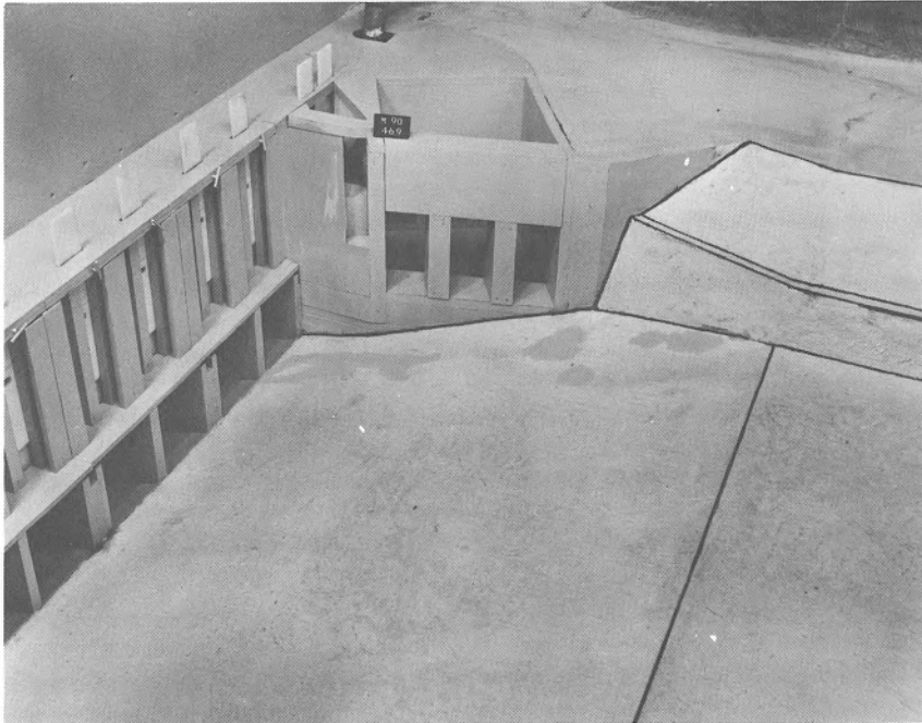
Fig. 6. General view of plan F south fishway entrance and plan H powerhouse intake (final designs).
