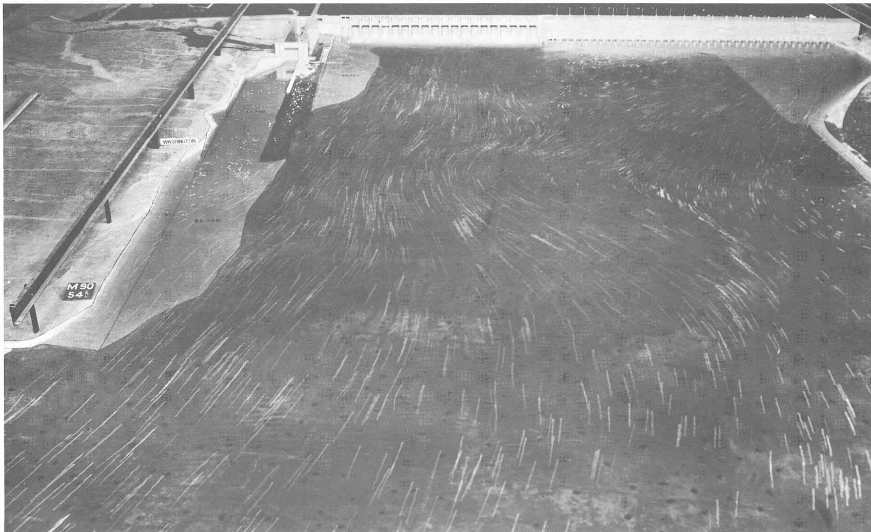
Photograph 30. Flow patterns downstream from final design structures; river discharge 800,000 cfs; powerhouse discharge 234,000 cfs, units 1 to 10; spillway discharge 563,075 cfs, uniformly distributed among bays 2 to 20, 2700 cfs through bay 1; fishway flow 225 cfs.
