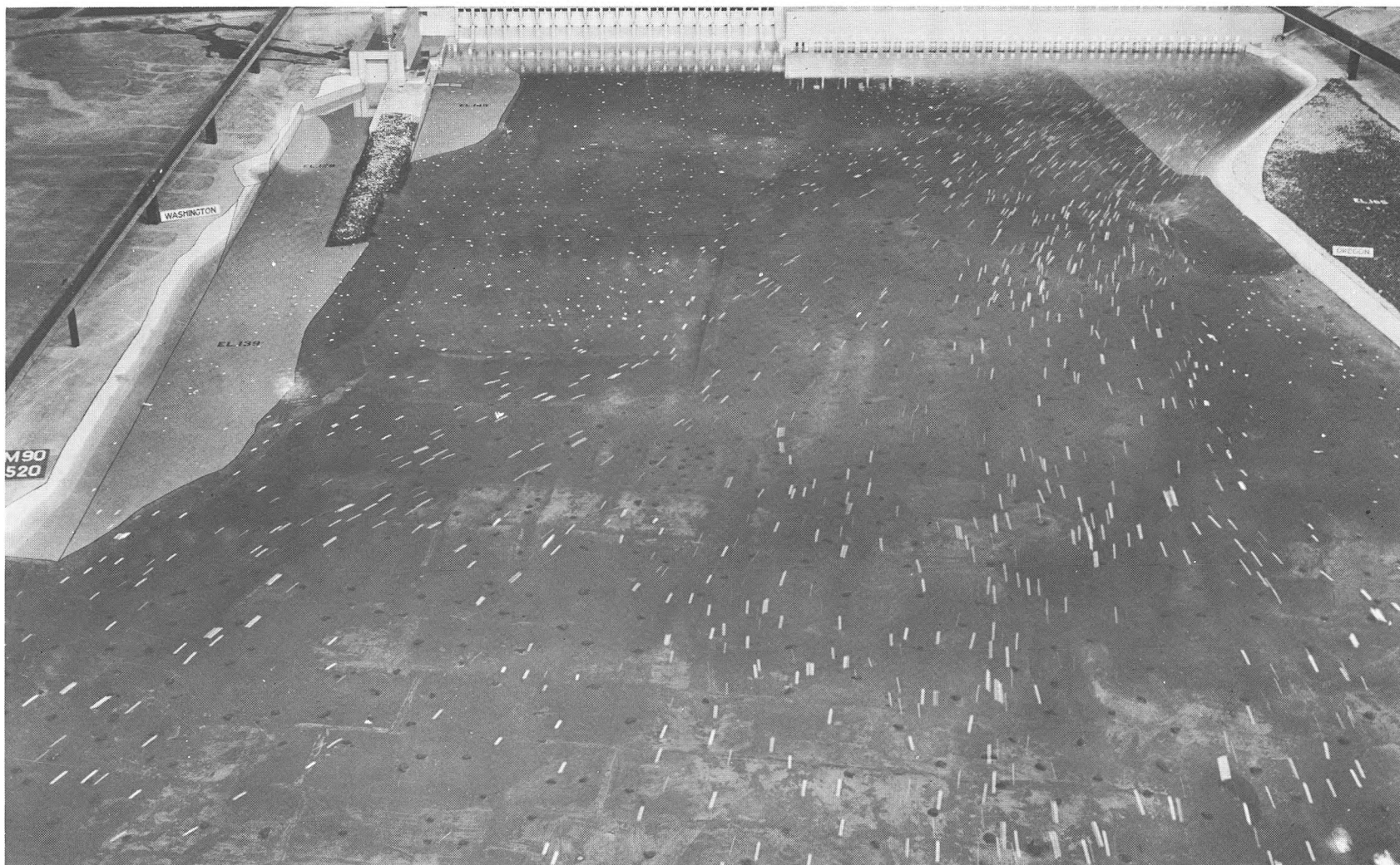
Photograph 23. Flow patterns downstream from final design structures; river discharge 200,000 cfs; powerhouse discharge 199,775 cfs, units 1 to 10; spillway closed; fishway flow 225 cfs.
