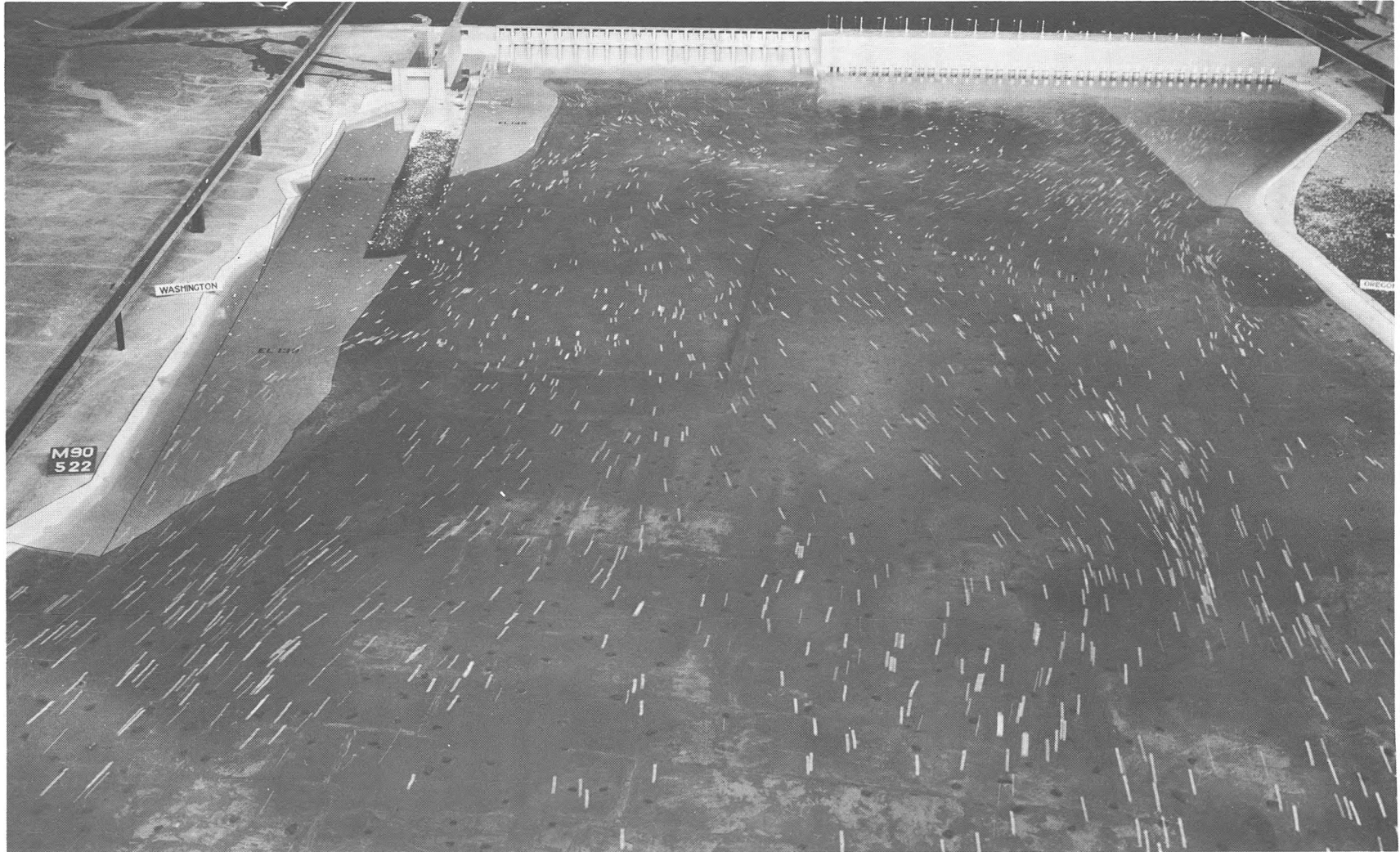
Photograph 24. Flow patterns downstream from final design structures; river discharge 400,000 cfs; powerhouse discharge 214,000 cfs, units 1 to 10; spillway discharge 183,075 cfs, uniformly distributed among bays 2 to 20, 2700 cfs through bay 1; fishway flow 225 cfs.
