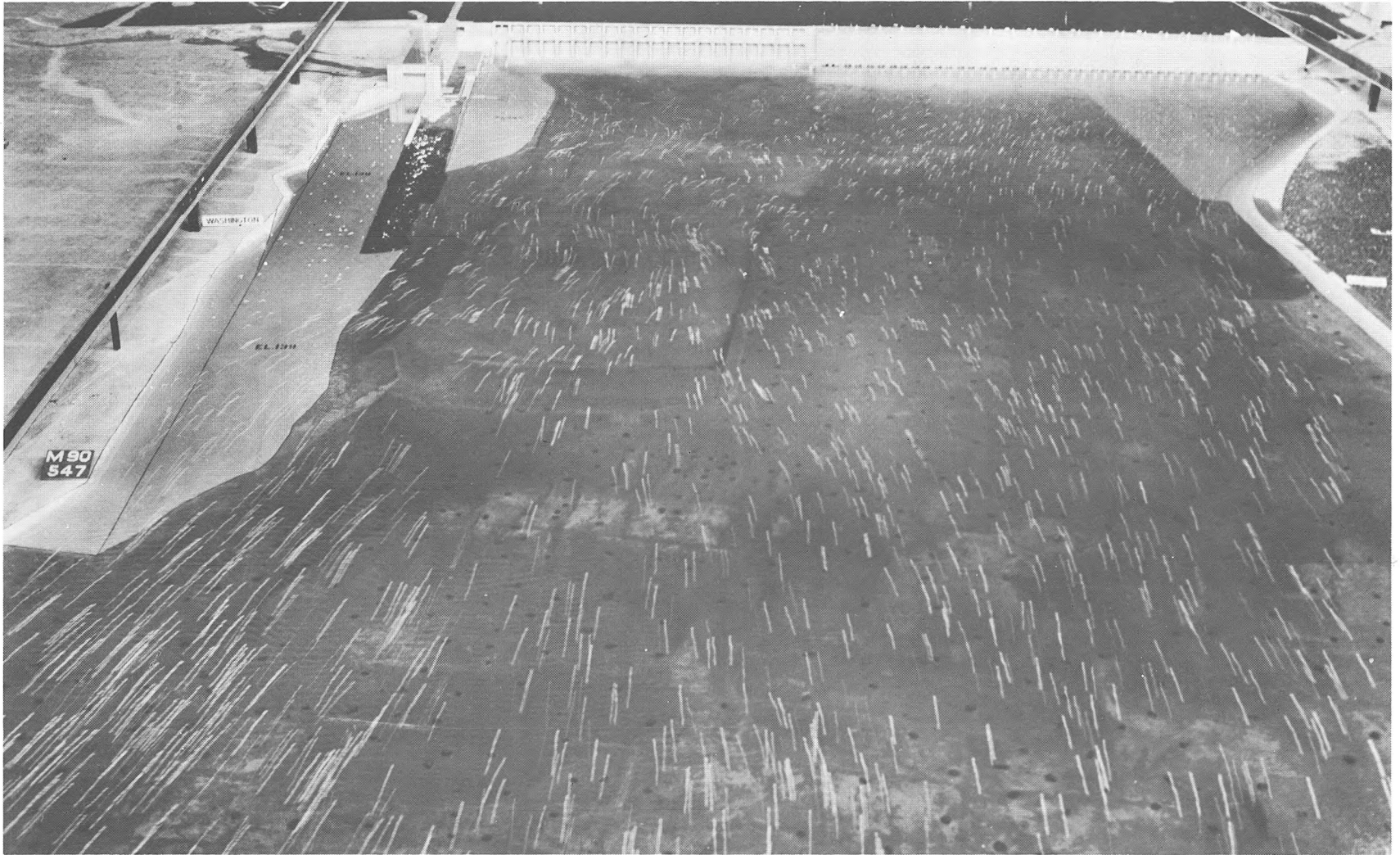
Photograph 31. Flow patterns downstream from final design structures; river discharge 800,000 cfs; powerhouse discharge 468,000 cfs, units 1 to 20; spillway discharge 329,075 cfs, uniformly distributed among bays 2 to 20, 2700 cfs through bay 1; fishway flow 225 cfs.
