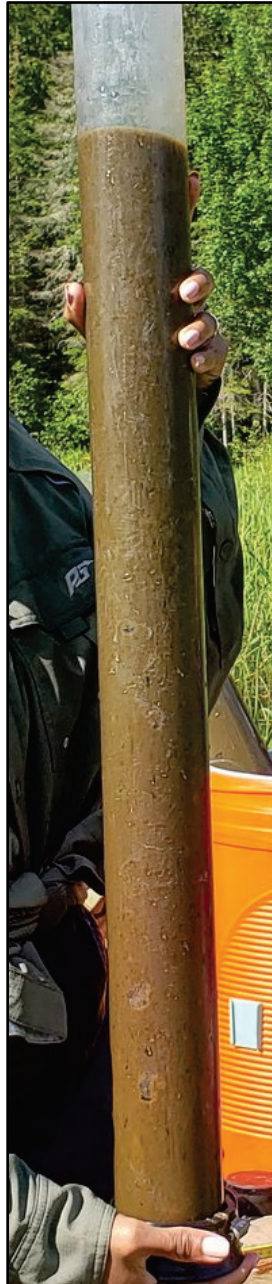
Figure 7. Soil core profile of the organic, mucky substrate often associated with wildrice stands.
