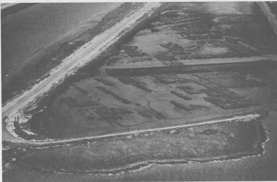
SALT POND 3. A study of marsh development on confined dredged material in an abandoned 10-acre salt pond in South San Francisco Bay demonstrated that a Spartina foliosa marsh can be established within 2 years. Aspects of plant spacing, substrate preparation, plant elevation, planting season, planting efficiency, and natural colonization were explored; cost estimates were prepared for the various
