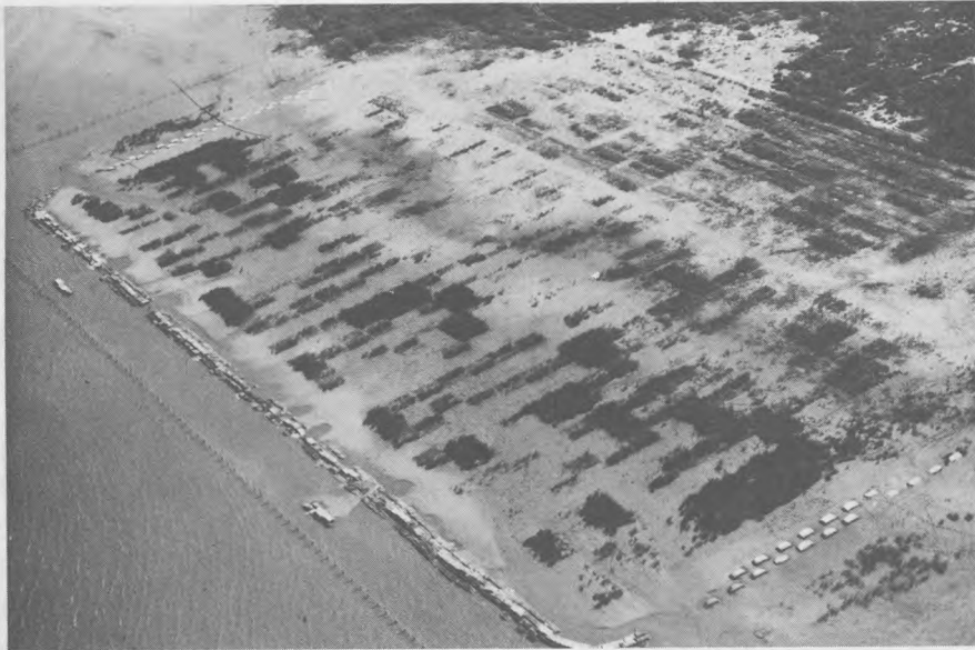
SALT POND 3. A study of marsh development on confined dredged material in an abandoned 10-acre salt pond in South San Francisco Bay demonstrated that a Spartina foliosa marsh can be established within 2 years. Aspects of plant spacing, substrate preparation, plant elevation, planting season, planting efficiency, and natural colonization were explored; cost estimates were prepared for the various
