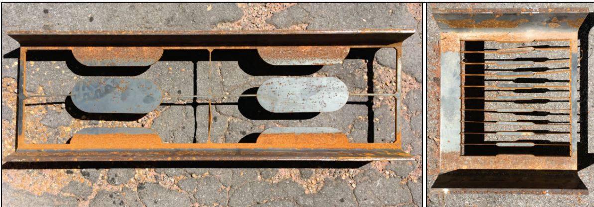
Figure 2. Sections of the S12 × 31.8 beam after dynamic ( left ) and static ( right ) specimens were cut from the web.
