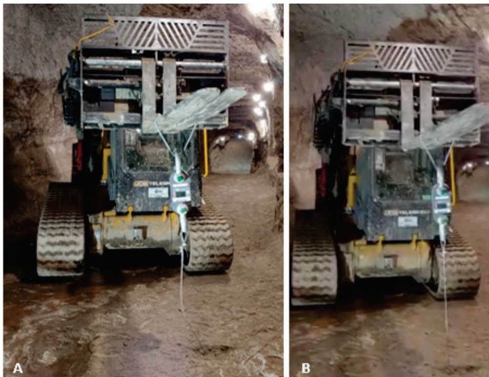
Figure 4-8 Cable attached to forklift via dynamometer: (A) slack; (B) tensioned.
