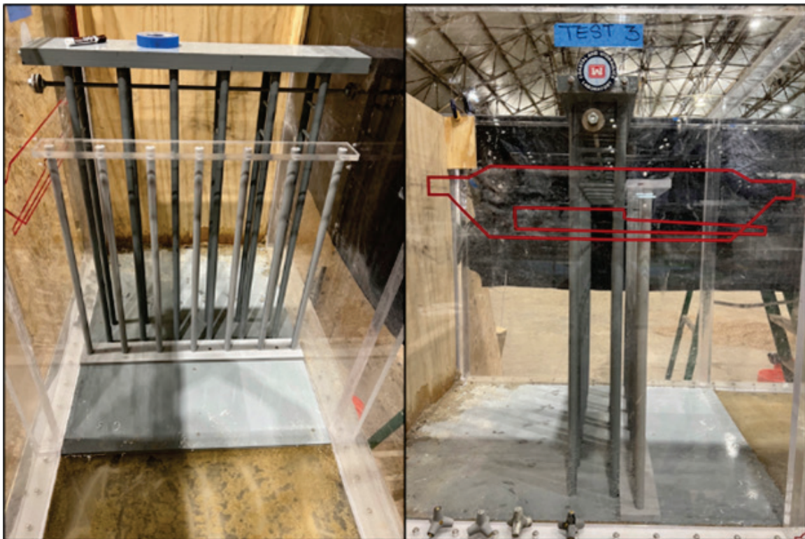
Figure 24. Placement of third row of piles downstream of bridge: front ( left ) and side ( right ) views.
