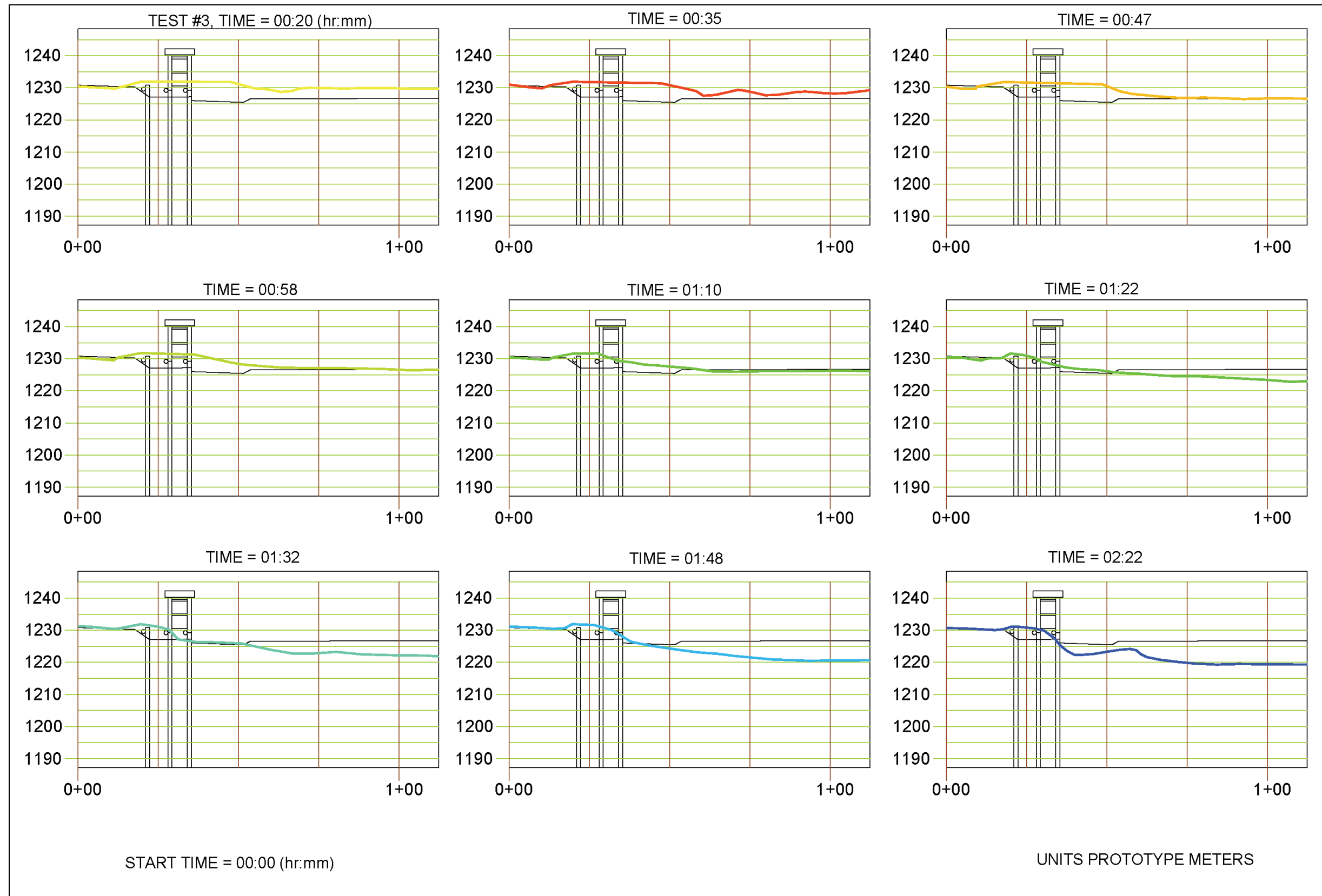
Figure 48. Scour profiles of model alternative 3.
