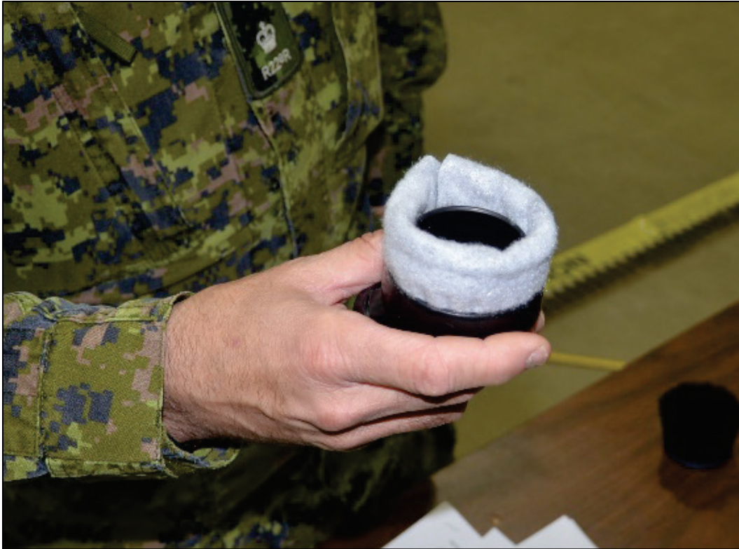
Figure 21. Photo of suggested modification to the brush end of the HEPA vacuum. This prototype uses a FiberTect wipe as the brush tip. Image is from the AE/P-22 operational assessment.
