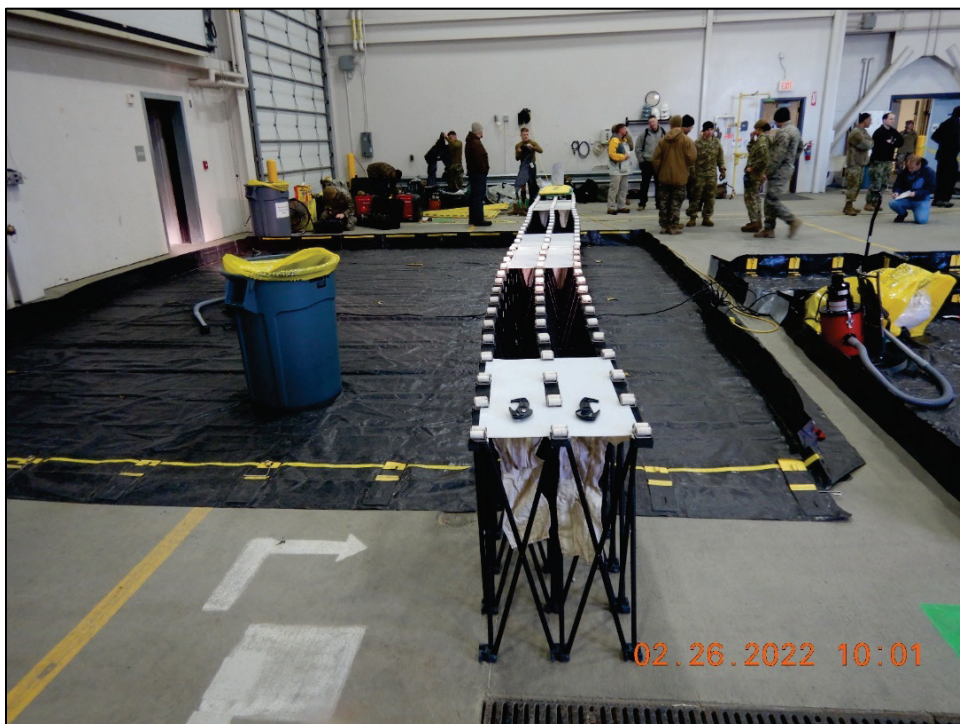
Figure 14. View of the decontamination line from the hot , or approach, side at AE/P-22. Nonambulatory on the right , ambulatory on left . Wastebaskets are provided for disrobing contaminated garments.
