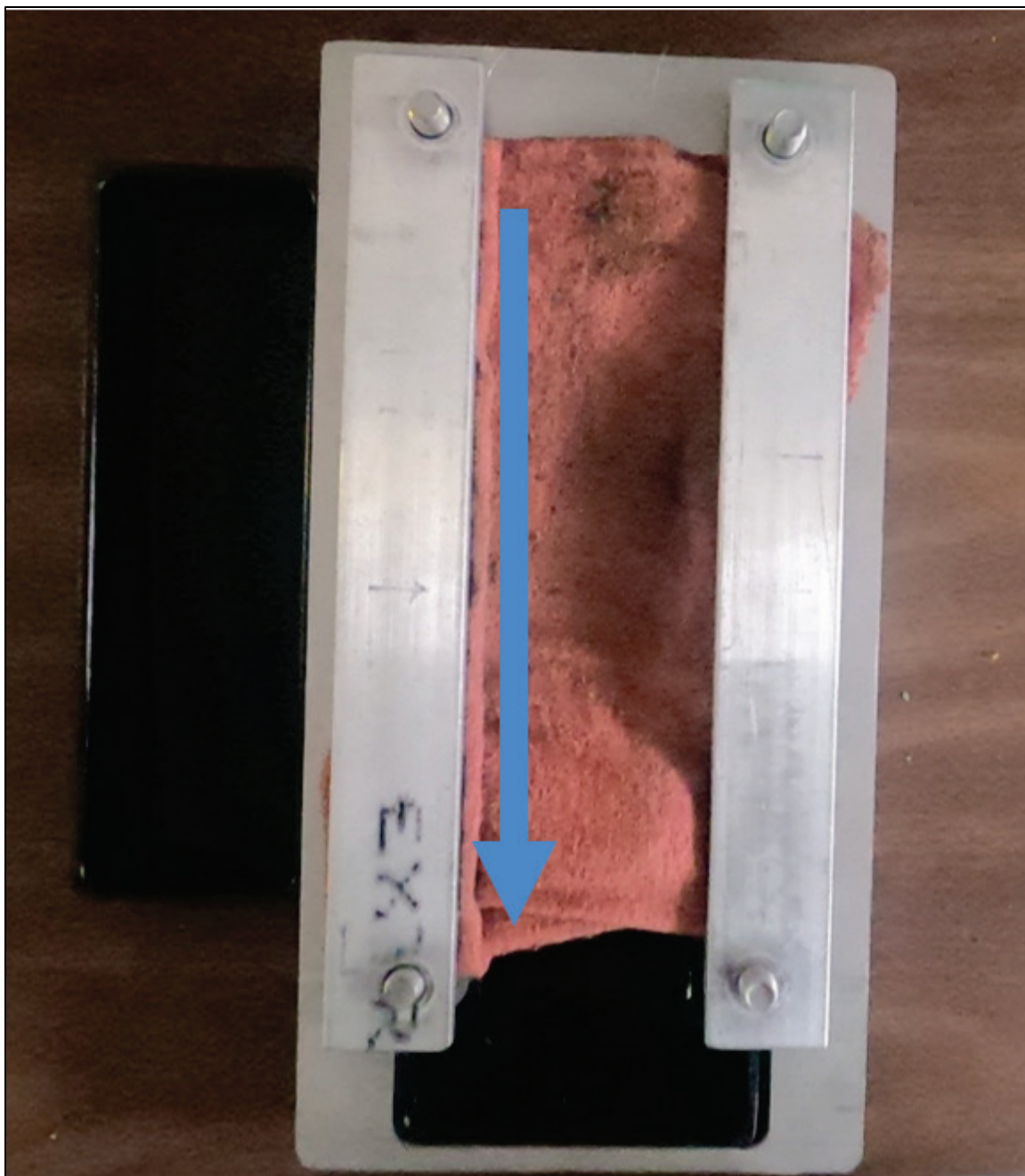
Figure 3. Sampling rig showing configuration with pig skin (nonrepresentative sample shown) for first stroke with FiberTect wipes.
