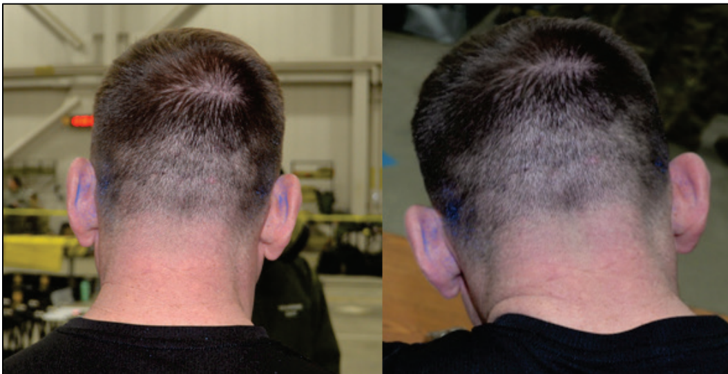
Figure 19. Before ( left ) and after ( right ) photo of a role player with blue simulant behind his ear. Decontamination was performed with 12 × 12 in. FiberTect wipes. Images are from AE/P-22 operational assessment.
