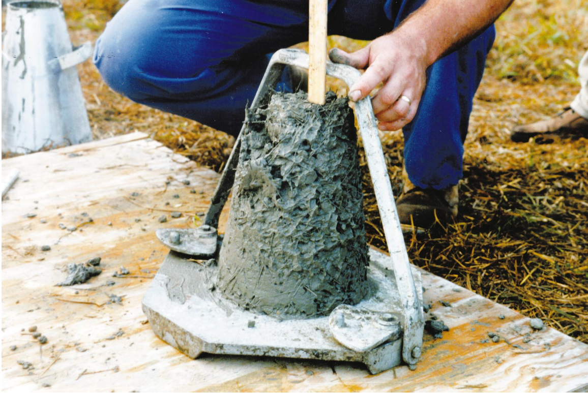
Figure 43. Typical slump of polyolefin FRC placed in USAEWES whitetopping section
