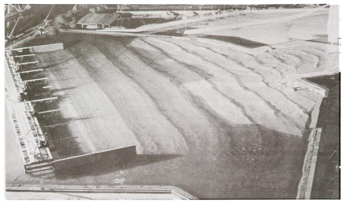
State-of-the-art electrohydraulic wave generator
