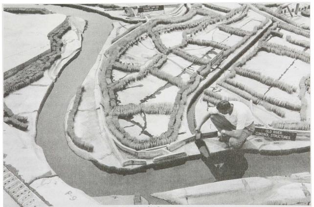
Portion of Mississippi River Flood Control model showing Old River control structures
