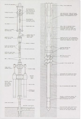
Rotary cone penetrometer designed by Hvorslev
