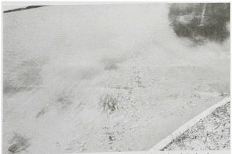
Oat grains provided a convenient material to simulate bed materials
