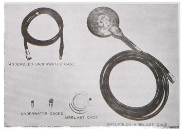
Instrumentation developed by WES for underwater blast tests
