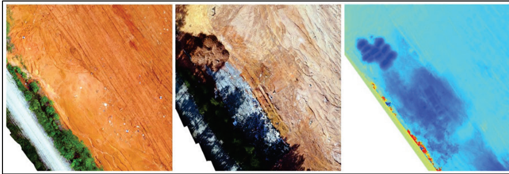
Figure 6. The images are from June ( left ), October ( middle ), and elevation difference ( right ) and feature a portion of the active cell at Gibson Road Landfill, as seen from the northern direction.
