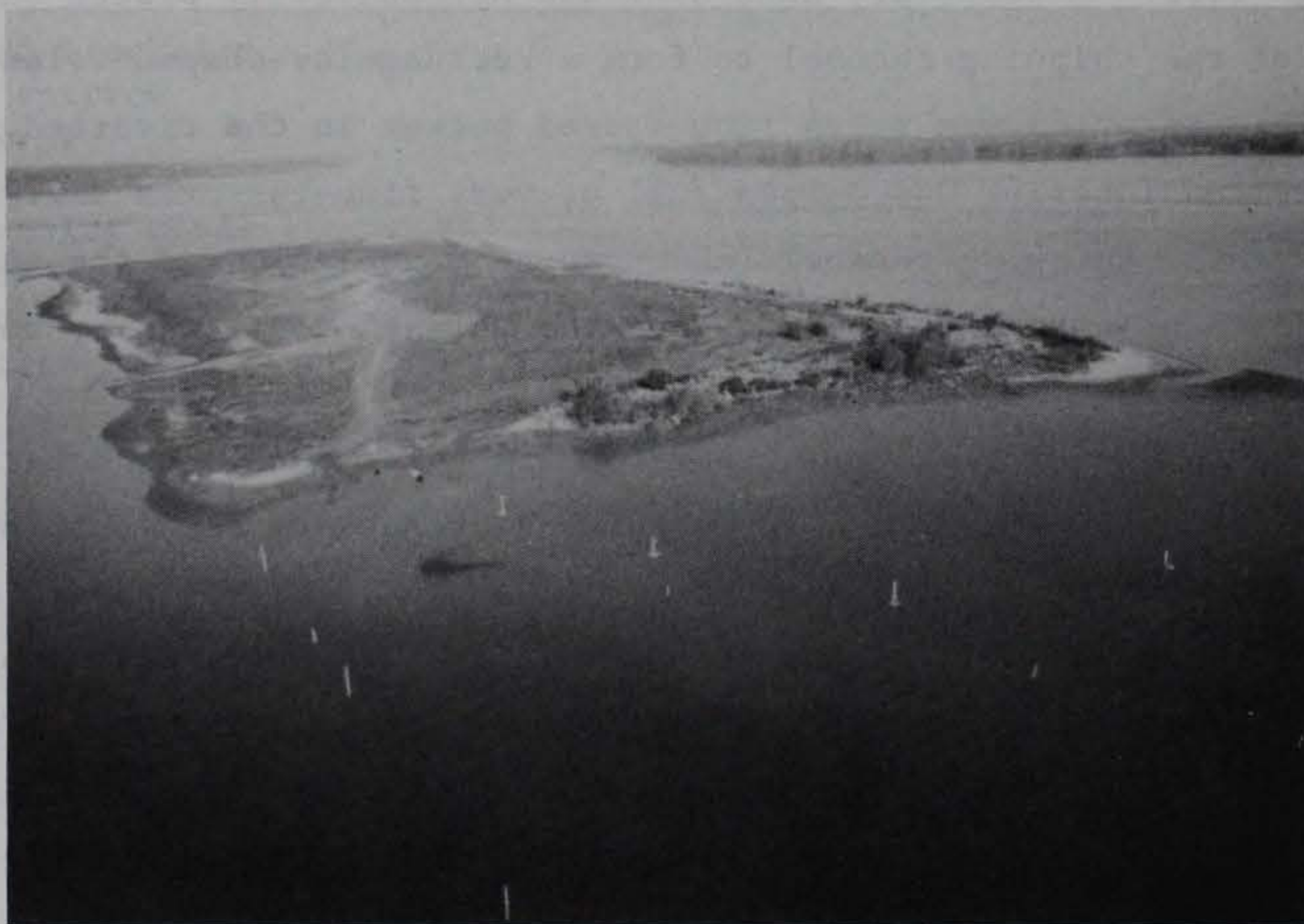
Figure 20. The WP site 3 years after the sand dike and silty dredged material had been placed to form the island, showing interior wetland vegetation development
