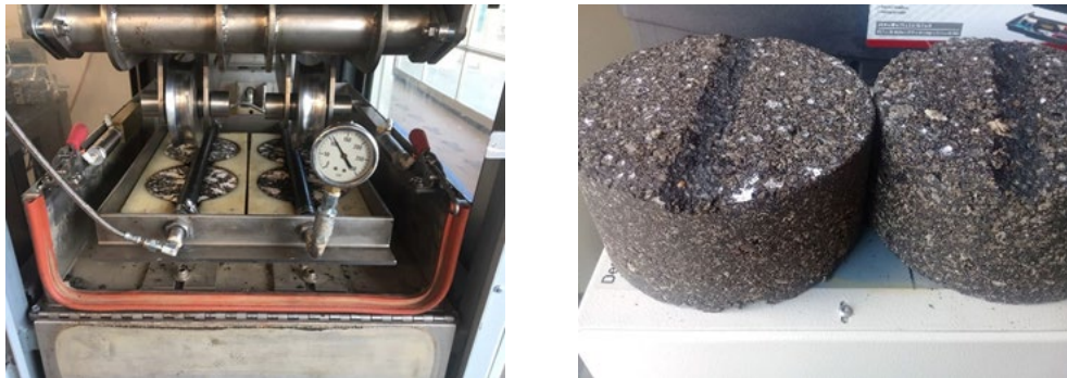
Figure 15. Asphalt pavement analyzer test.
