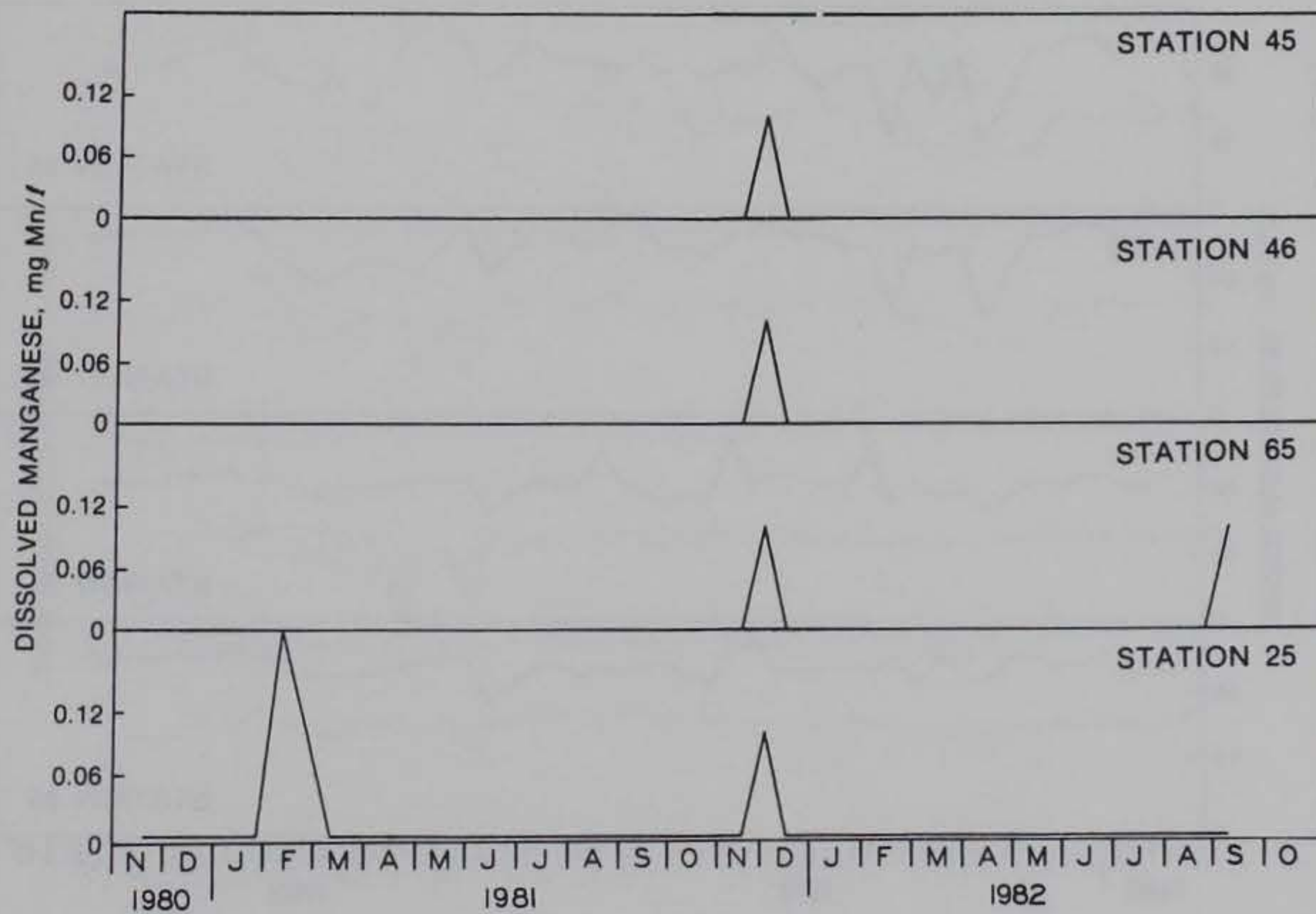
Figure B20. Changes in dissolved manganese in the tributary sampling stations, November 1980-September 1982
