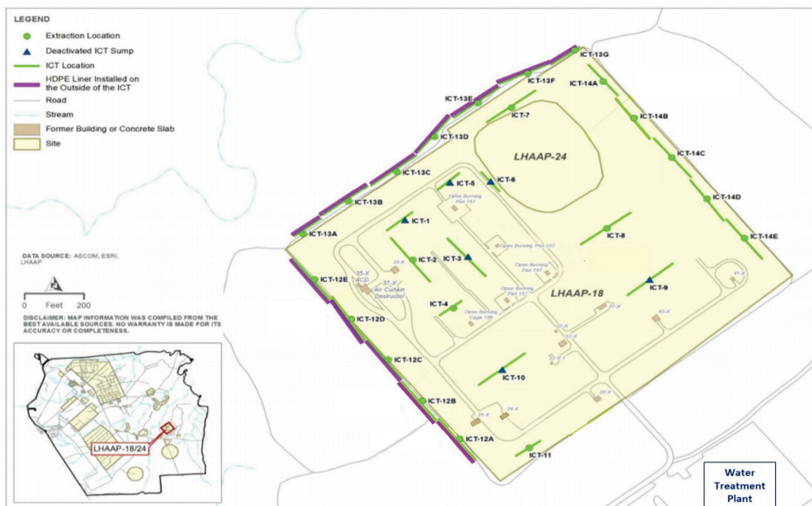
Figure 1. Map of LHAAP showing operable units LHAAP-18/24 and the associated interception trenches which feed the GWTP*.
