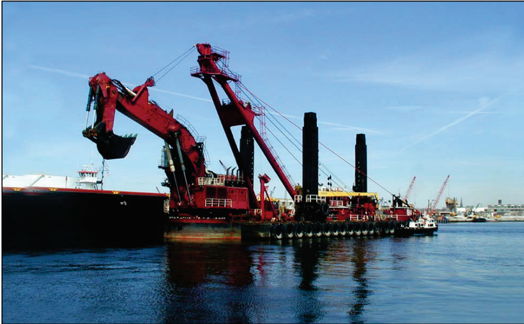
Figure 4. Mechanical (backhoe) dredge.
