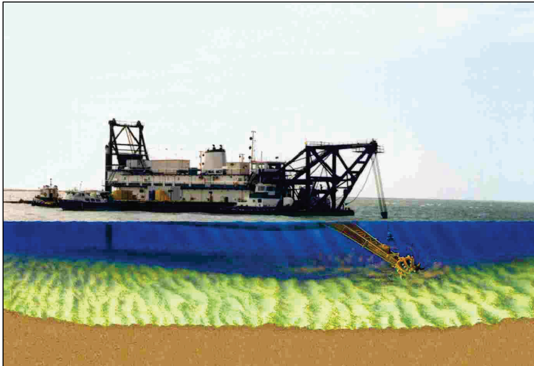
Figure 1. Hydraulic cutterhead pipeline dredge.
