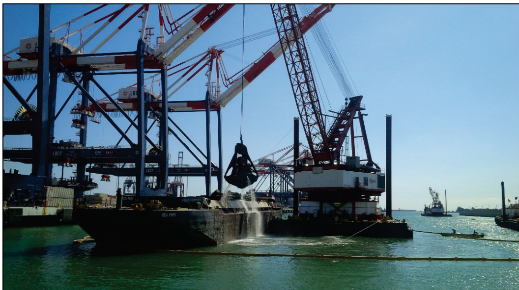
Figure 9. Clamshell dredge loading steel (grizzly) barge screen at Port of Long Beach, CA (Hoffman et al. 2015)
