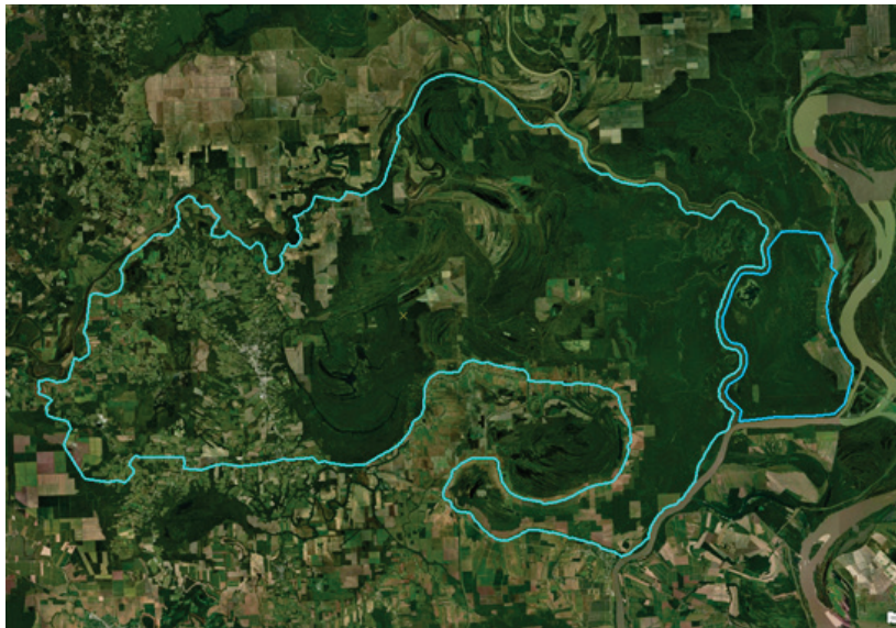
Figure 1. RAS terrain showing the spatial extent of the 2D flow areas and the cross sections for the 1D reaches.
