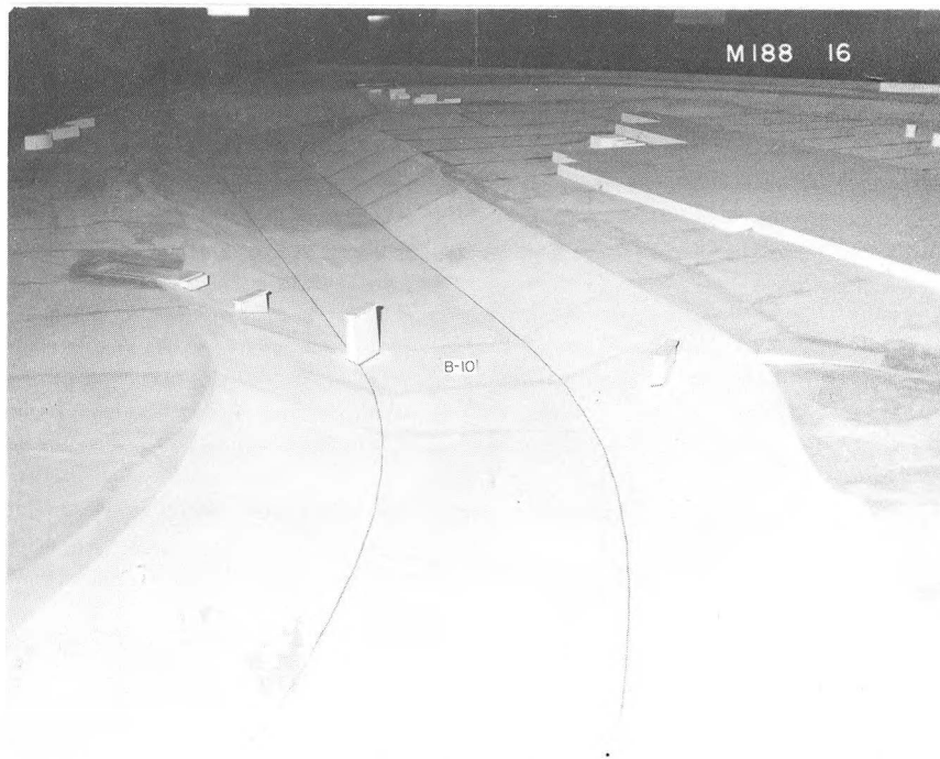
Photograph 2. Bridge B-10 and adjacent channel Electric furnace building in background (upper right) (Before final roughness adjustment for verification)
