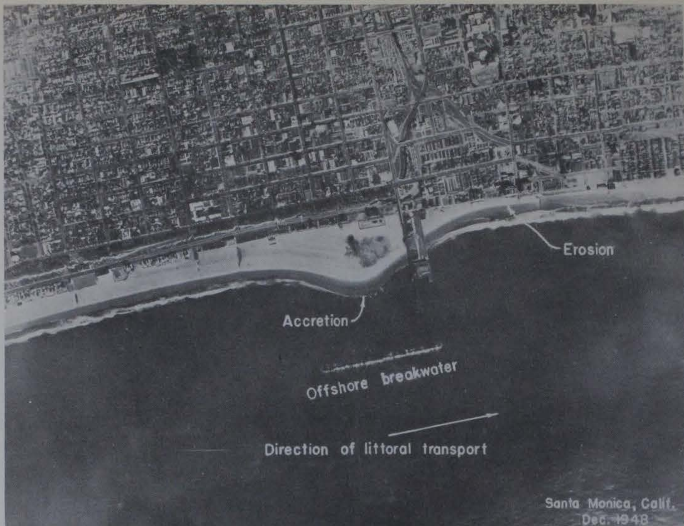
FIGURE 48 EFFECT OF OFFSHORE BREAKWATER
