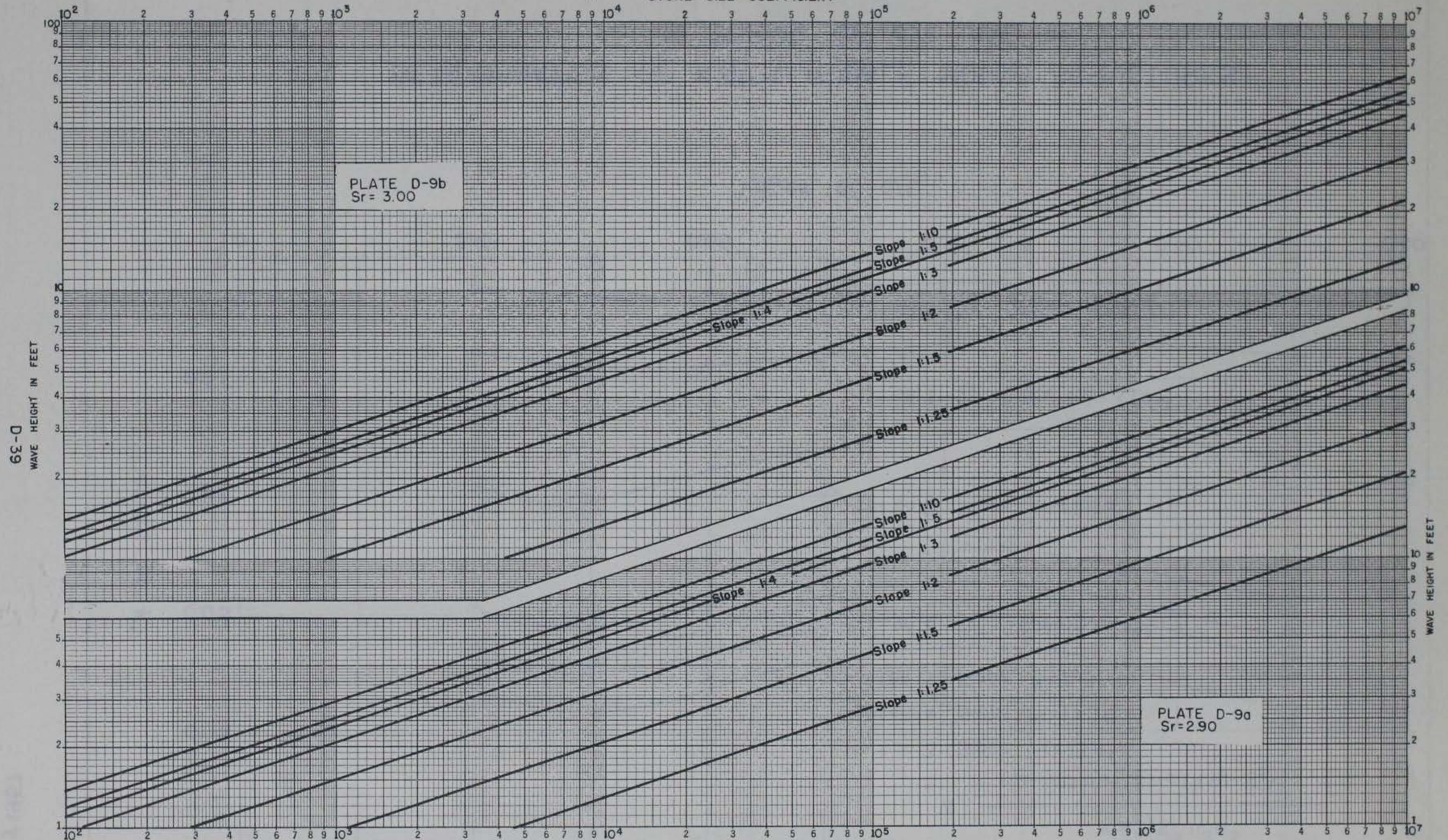
STONE WEIGHT VS WAVE HEIGHT FOR VARIOUS VALUES OF BREAKWATER SLOPE (Sr=2.90 & Sr=3.00) PLATE D-9
