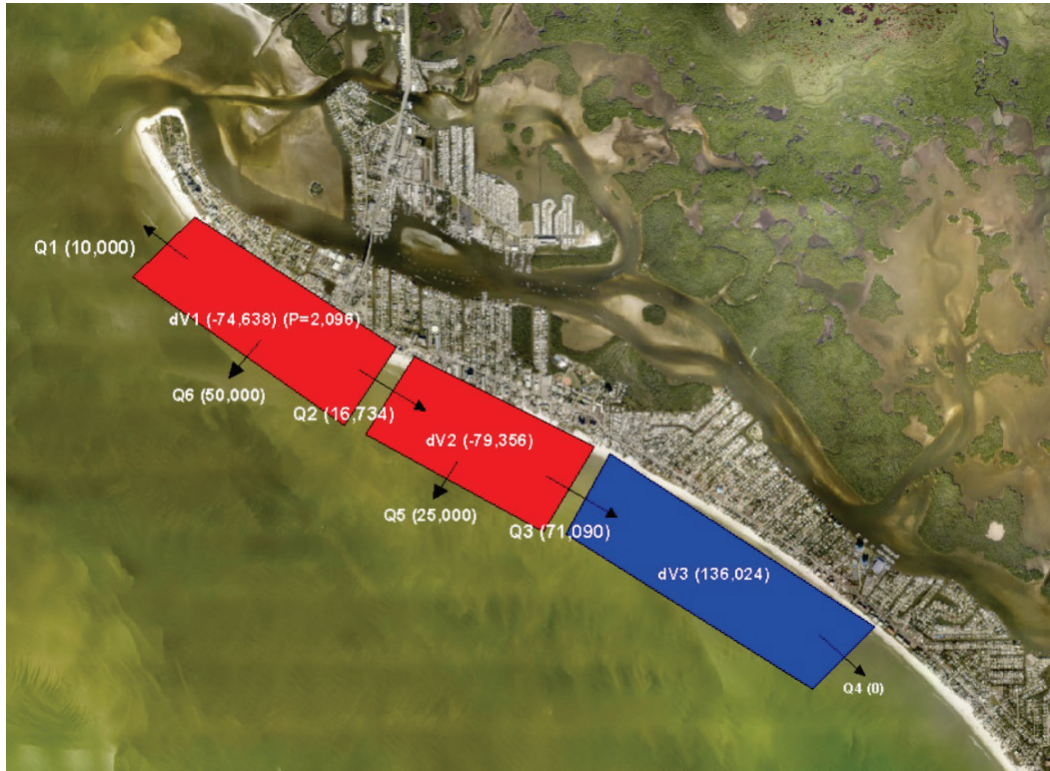
Figure 30. Results of a sediment budget calculation based on net sediment volume changes measured in the control areas and berm areas between August 2016 and January 2018. Measured volume changes are in cubic yards (dV) and calculated transport values in cubic yards per year (Q) .
