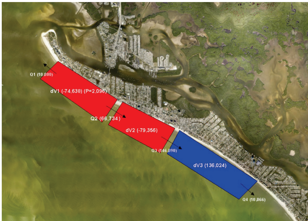
Figure 29. Results of a sediment budget calculation based on net sediment volume changes measured in the control areas and berm areas between August 2016 and January 2018. Measured volume changes are in cubic yards (dV) and calculated transport values in cubic yards per year (Q) .
