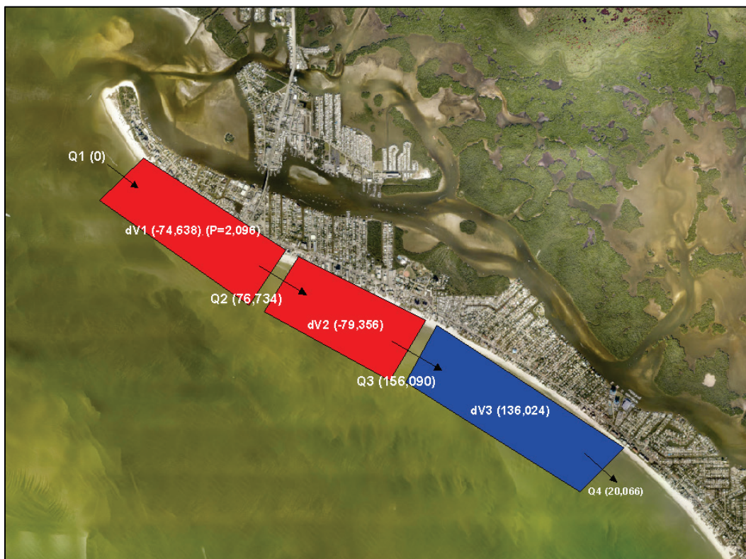
Figure 28. Results of a sediment budget calculation based on net sediment volume changes measured in the control areas and berm areas between August 2016 and January 2018. Measured volume changes are in cubic yards (dV) and calculated transport values in cubic yards per year (Q) .
