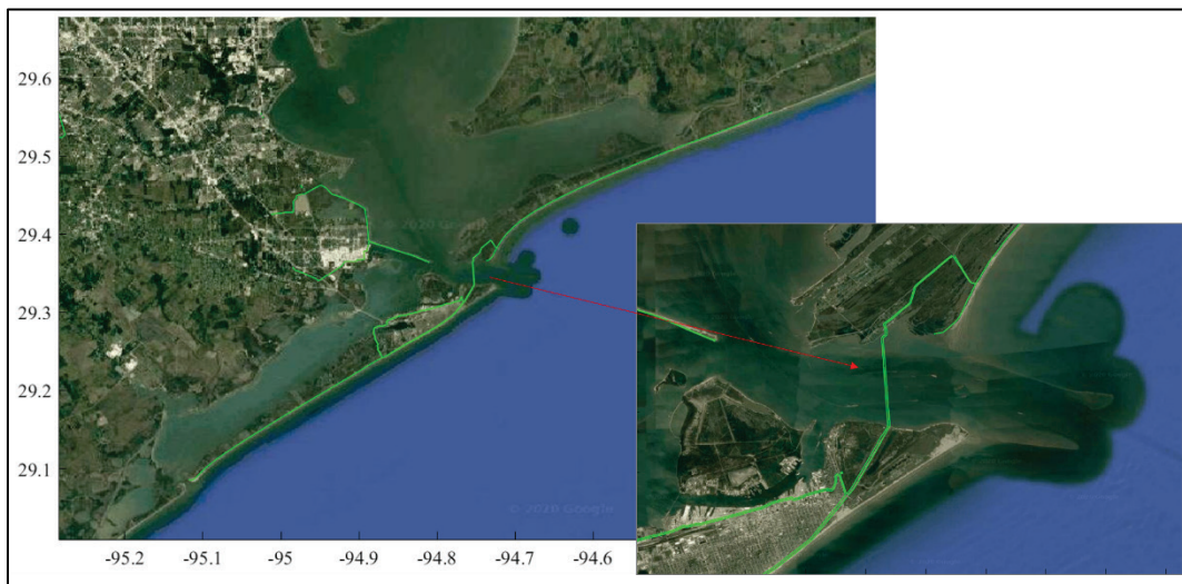
Figure D-11. Map showing the ADCIRC model representation of the full beach dune and gate system, labeled as BD_Alt6.
