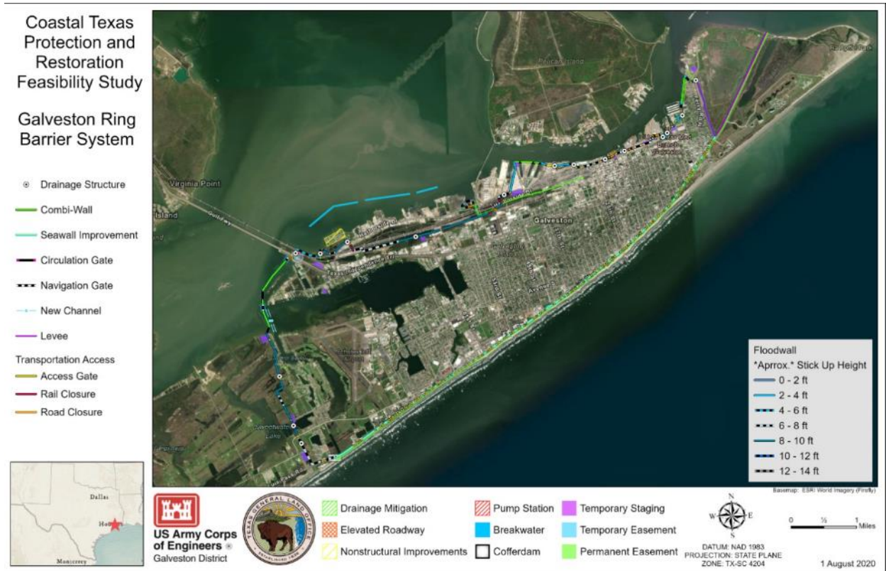
Figure 4-12: Galveston Ring Barrier System
