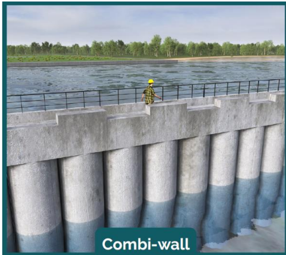
Figure 6-5: Combi-wall (Conceptual Rendition)
