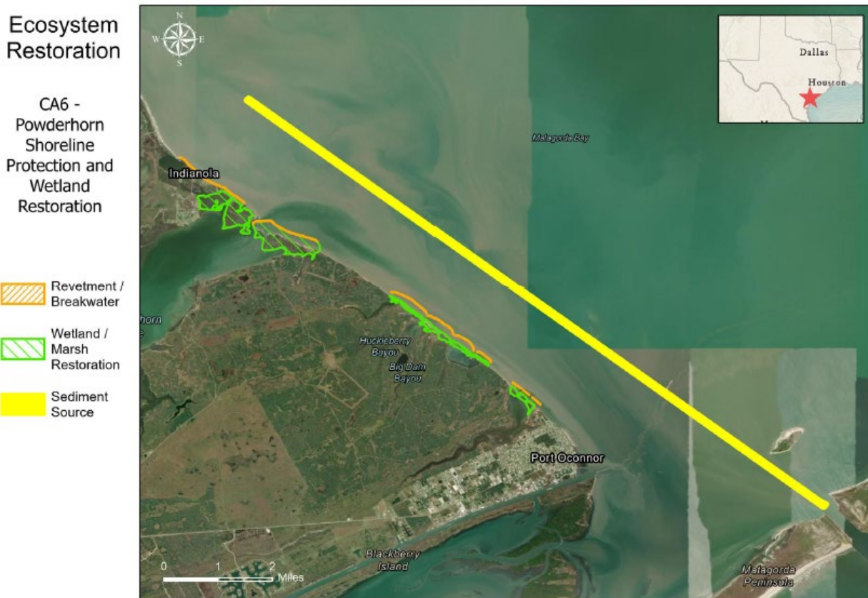
Figure 7-6: CA6 – Powderhorn Shoreline Protection and Wetland Restoration
