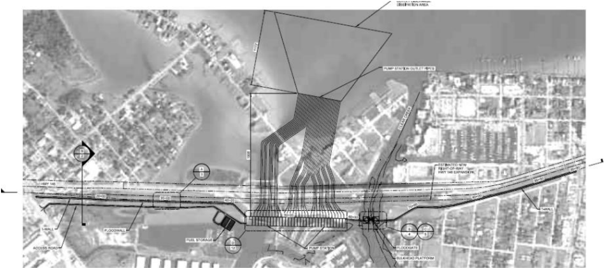
Figure 2-53: Clear Lake Gate System with Pump Station Footprint (Annex 7 has details).
