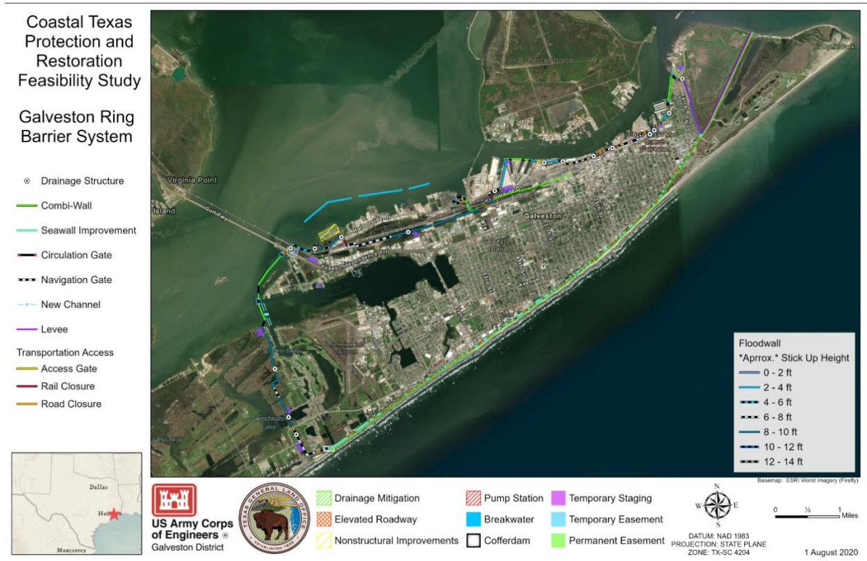
Figure 5.2: Galveston Ring Barrier System
